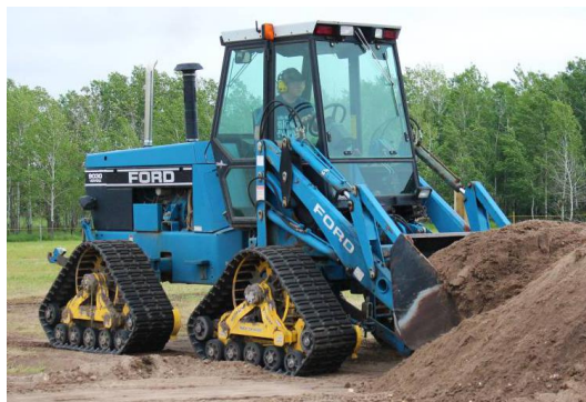
Figure 1. Engineering vehicle equipped with the track conversion system in operation.
