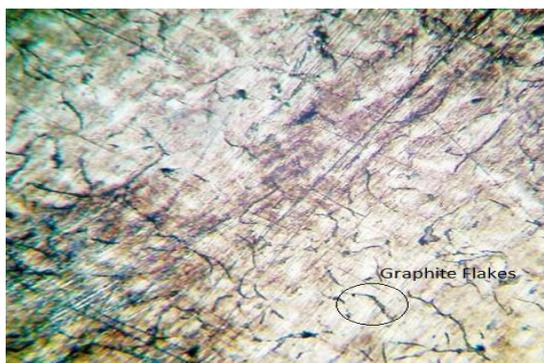
Figure 4. Micro-structure of GCI disc (Gray Cast Iron).
