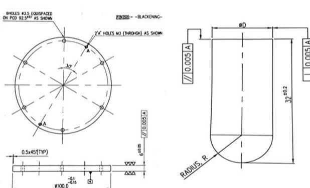
Figure 3. Sectional view of the disc and pin.
