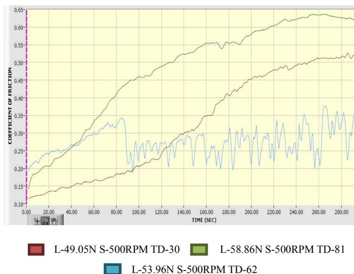
**Figure 6.** Variation and Comparison of Co-efficient of friction captured from Winducom software at constant Speed&different Load, Track diamter conditions [L-Load(N);S-Speed(Rpm)andTD-Trackdiamter(mm)].
