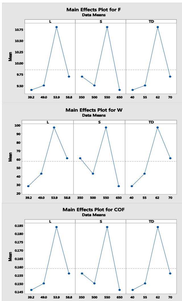
Figure 10. Main effects plot for Wear, Frictional force and Coefficient of friction for PTFE with Graphite material.
