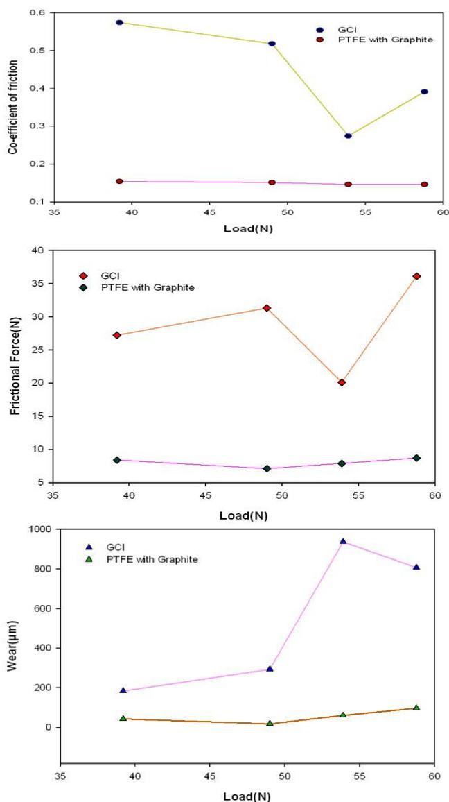
**Figure 7.** Variation of Wear, Frictional force and Co-efficient of friction with respect to Load for GCI and PTFE materials.
