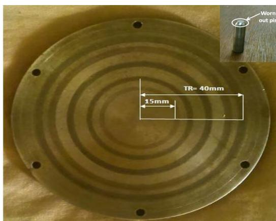
**Figure 5.** Photographic view of the Disc and Pin specimens used for experimentation and Track formation due to wear.
