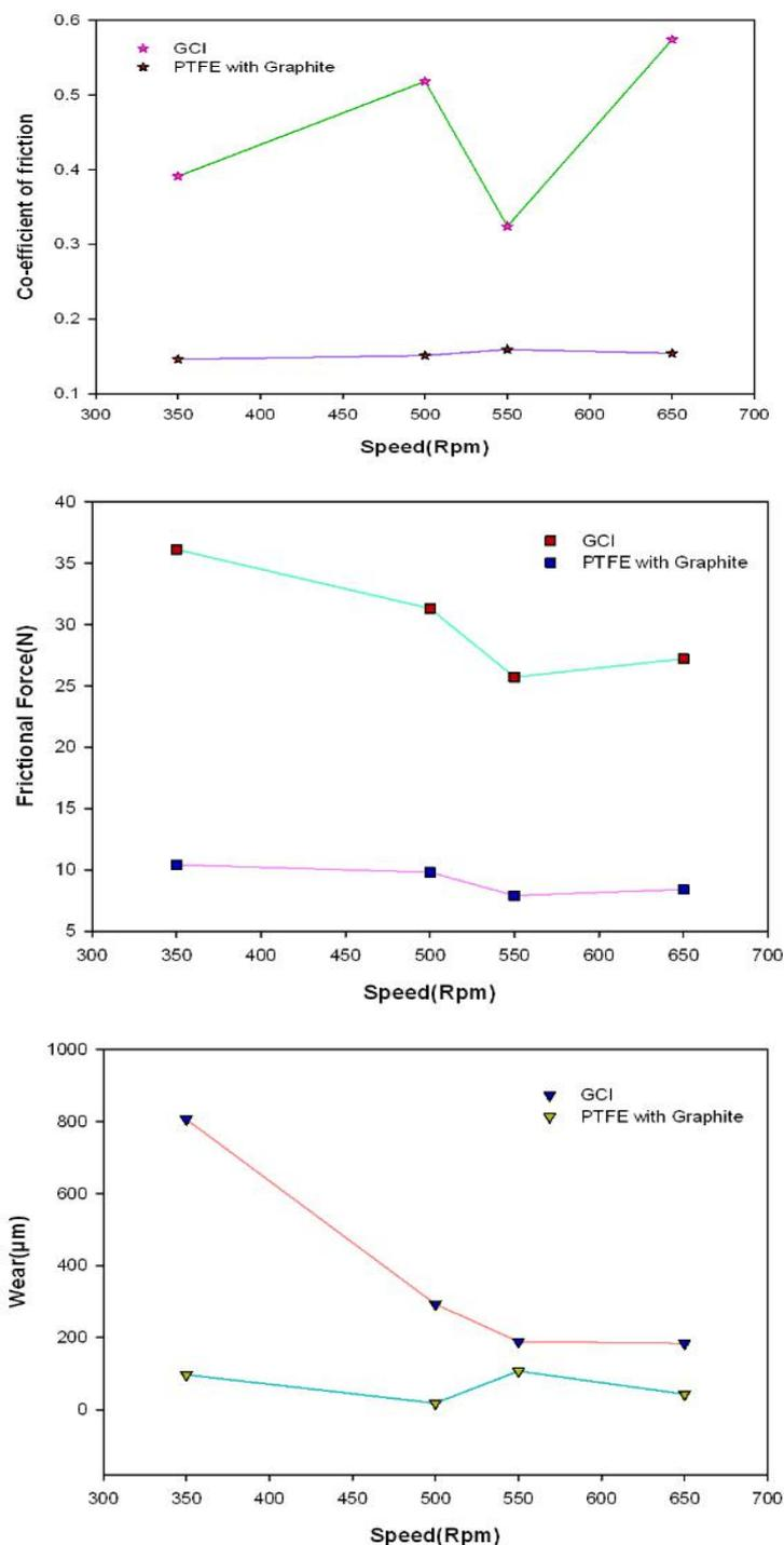
**Figure 8.** Variation of Wear, Frictional force and Co-efficient of friction with respect to Speed for GCI and PTFE materials.
