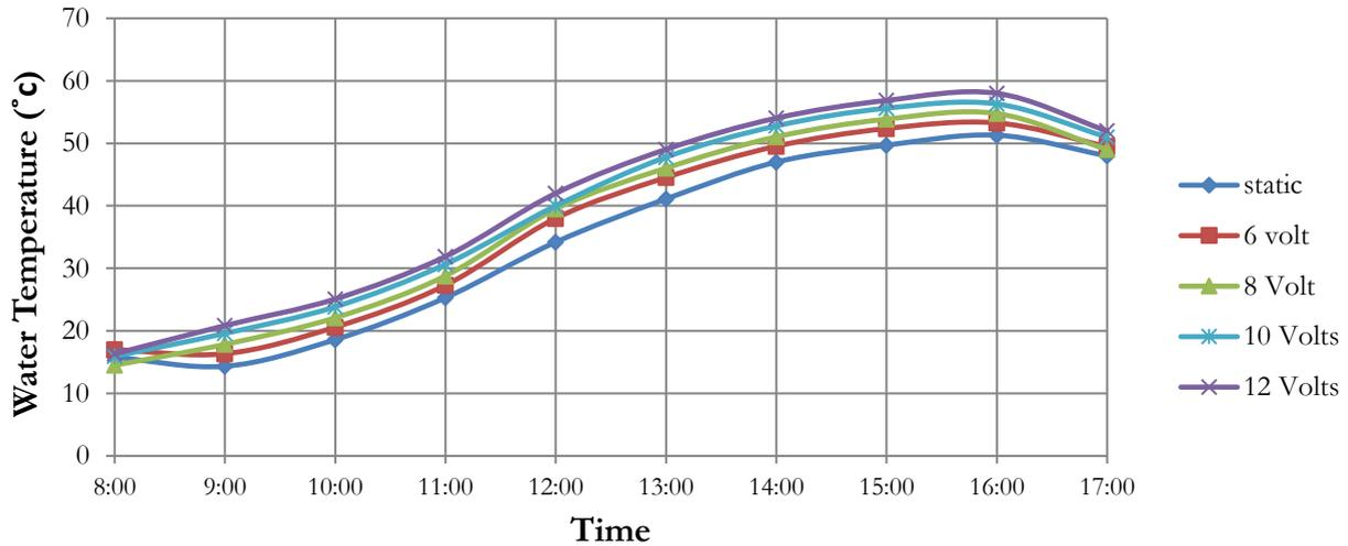
Figure 5. Mean water tank Temperature at various voltages
