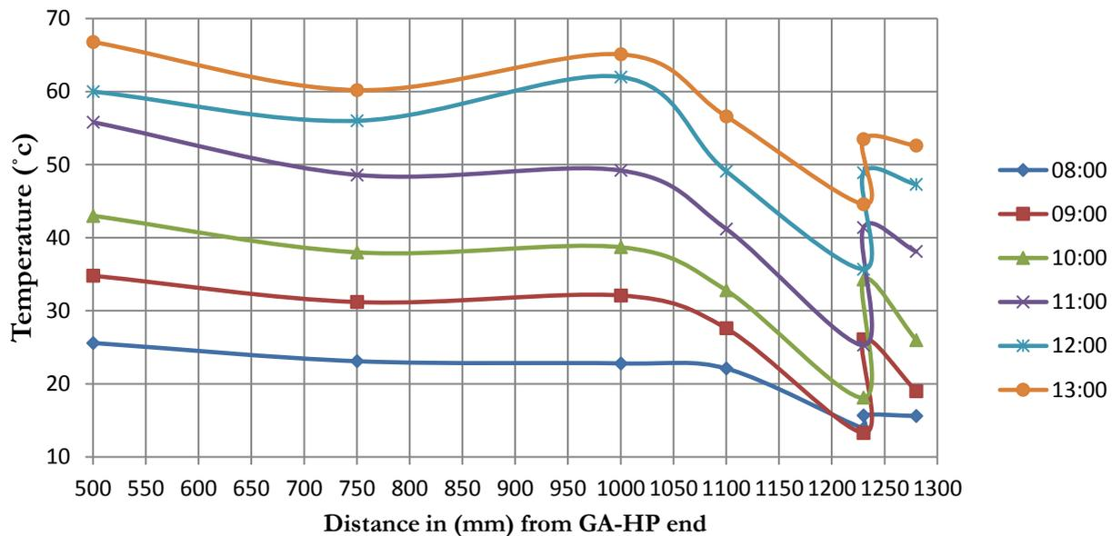
**Figure 7.** Temperature distribution along GA-HP with vibration
