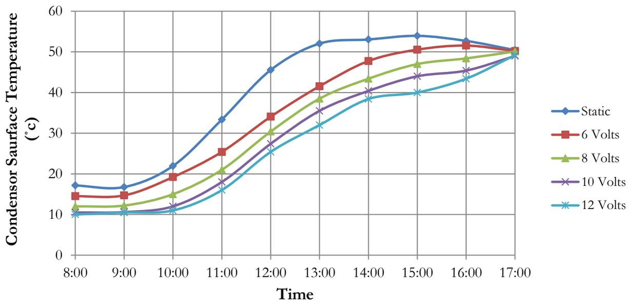
Figure 4. Mean surface Temperature of the condenser section of GA-HP at various voltages
