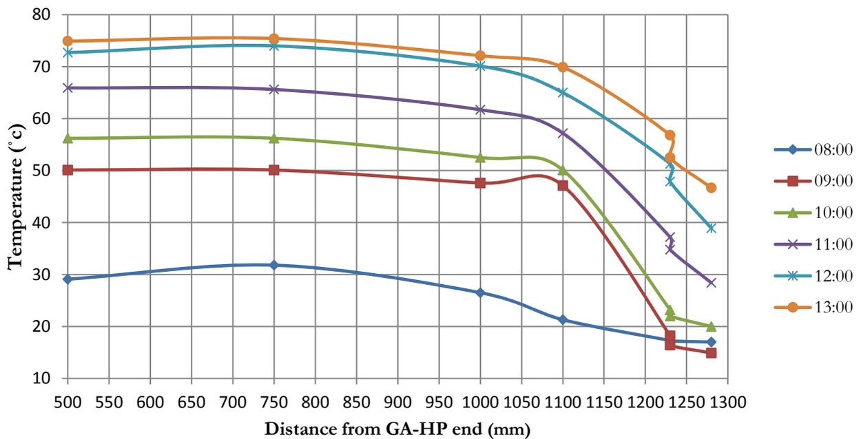
Figure 6. Temperature distribution along GA-HP without vibration
