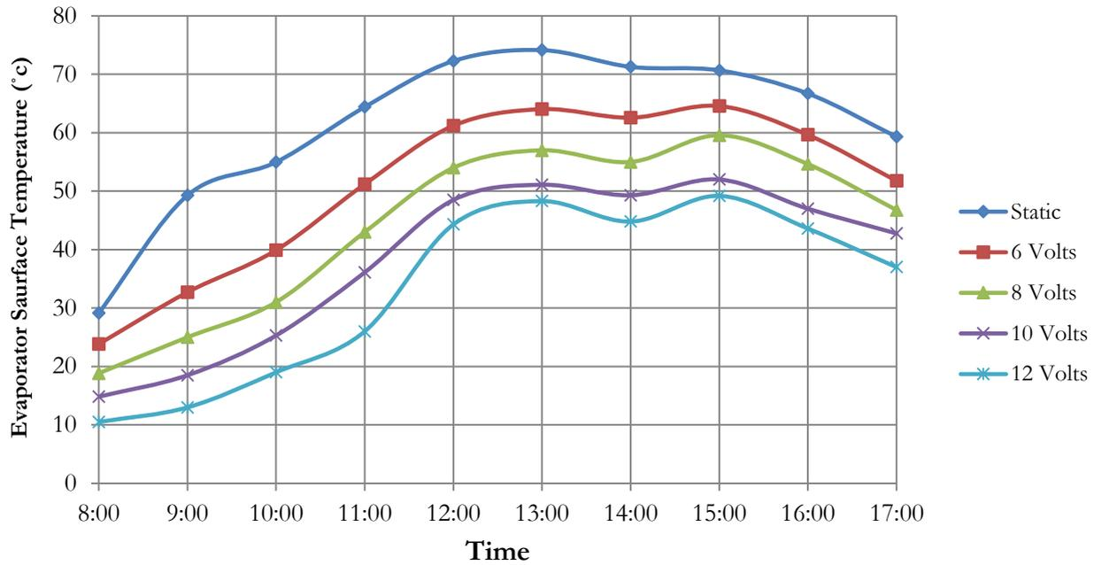
Figure 3. Mean surface Temperature of Evaporator Section of GA-HP at various voltages
