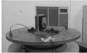
Figure 17. Two axes mirror libration test.
