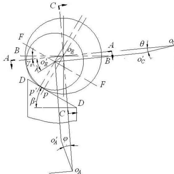
Figure 3. Geometric relation between roller and blade under normal condition.
