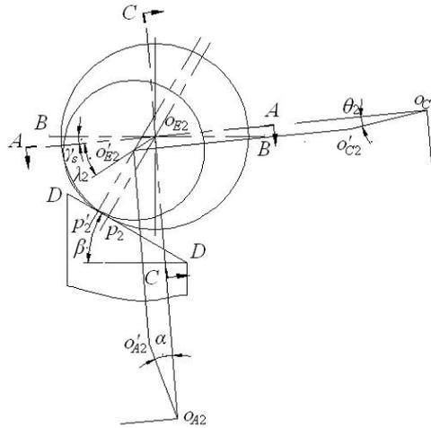
Figure 6. Roller-blade geometric relation under actual roller-grinding wheel relation.
