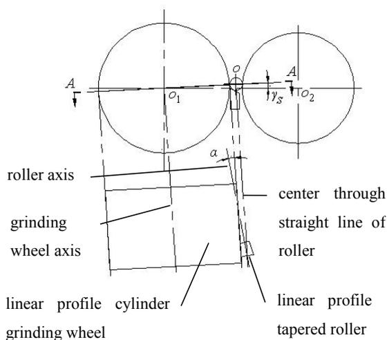
**Figure 2.** An ideal roller-grinding wheel relation in grinding linear profile roller by linear profile grinding wheel.
