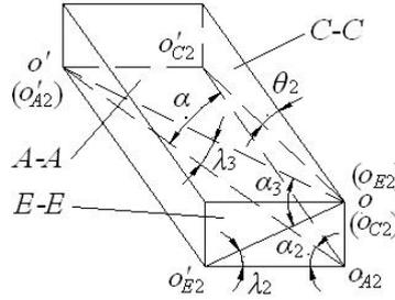
**Figure 7.** The geometric relation along roller axis direction under actual roller-grinding wheel relation.
