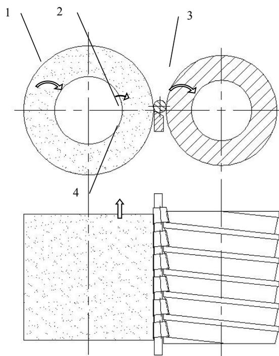
1—grinding wheel; 2—tapered roller; 3—guide wheel; 4—blade
