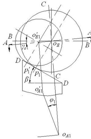
Figure 4. Roller-blade geometric relation when roller axis and grinding wheel axis are coplaned.
