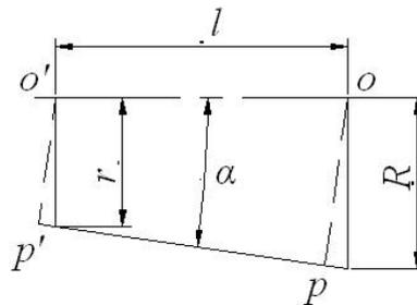
Figure 5. Relation between roller geometric parameters and distance from roller large/small end circle center to blade slope plane.
