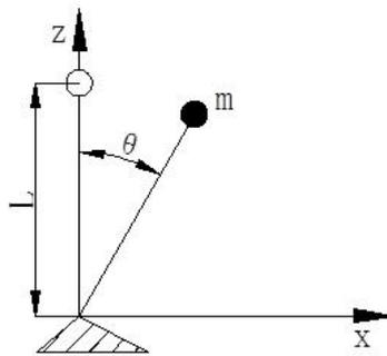
Figure 2. The inverted pendulum model of humanoid robot's forward motion.
