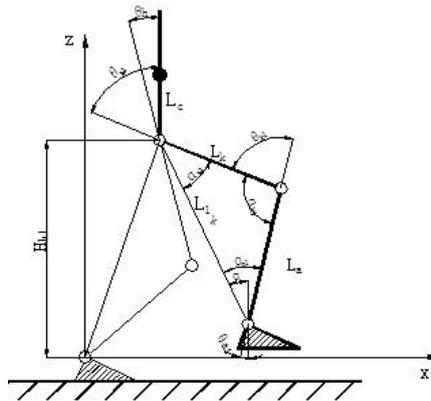
**Figure 8.** Geometry diagram of the humanoid robot's swing leg.
