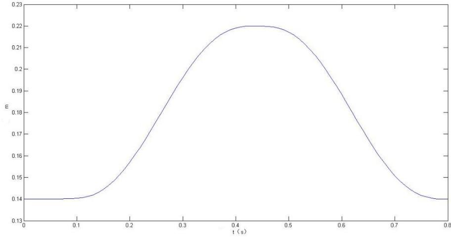
**Figure 6.** The motion trajectory of the swing leg in Z direction.
