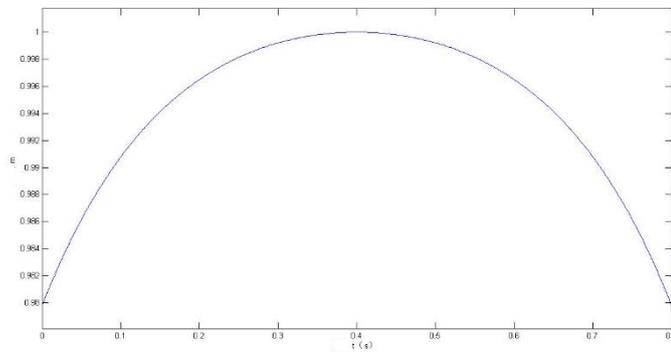
Figure 4. The motion trajectory of the humanoid robot centroid in Z direction.
