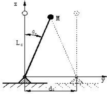
**Figure 9.** The inverted pendulum model of the robot centroid lateral movement.
