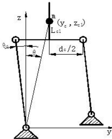
Figure 11. Schematic diagram of the lateral movement joint of humanoid robot.
