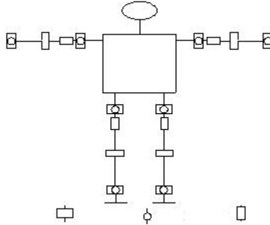
Figure 1. A humanoid robot model.
