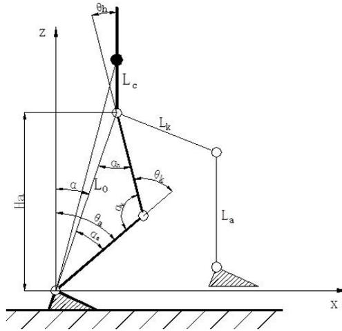
**Figure 7.** Geometry diagram of the humanoid robot's supporting leg.
