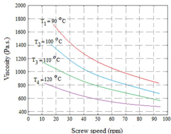
Figure 6. Viscosities against screw speed at various temperatures.
