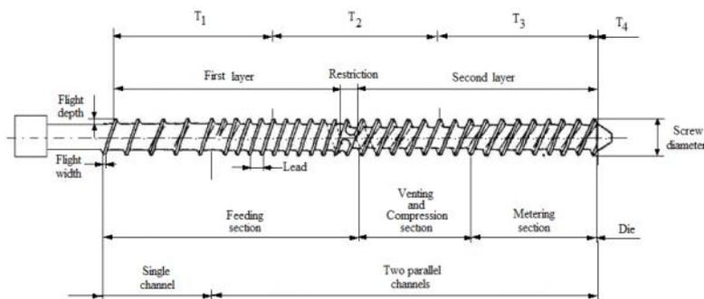
Figure 1b. Screw layers ( $T_1 = 90^\circ\text{C}$ ,  $T_2 = 100^\circ\text{C}$ ,  $T_3 = 110^\circ\text{C}$ ,  $T_4 = 120^\circ\text{C}$ ).
