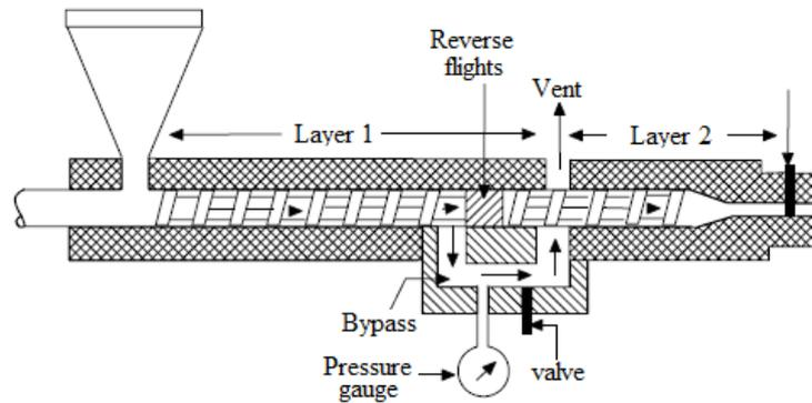
Figure 1a. Scheme of a two layer vented extruder with a valved bypass.
