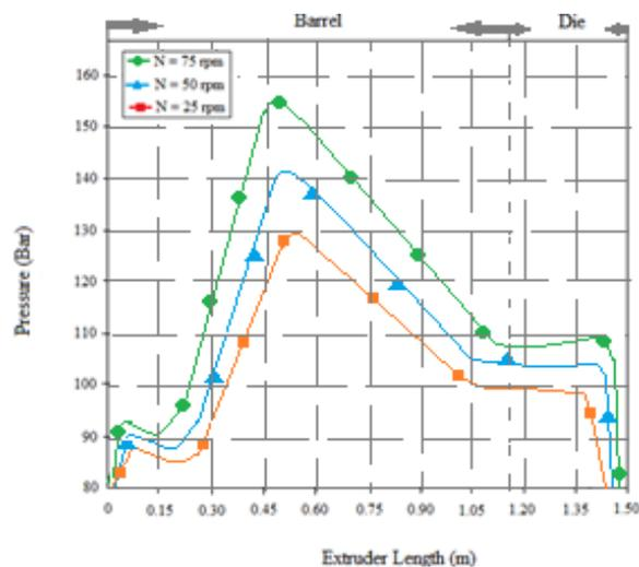
**Figure 4.** Variation of the pressure for three screw speeds in barrel and die.
