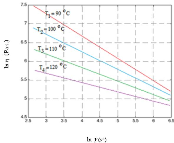
**Figure 3.** Values of  $\ln \eta$  against  $\ln \dot{\gamma}$  for PVC at the four temperatures.
