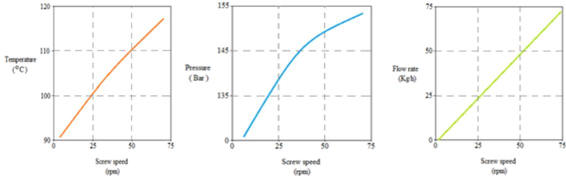
Figure 2. a) The temperature varies linearly with the screw speed; b) The pressure varies linearly with the screw speed; c) The flow rate varies linearly with the screw speed.
