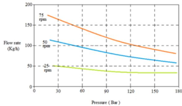
Figure 5. Variation of the flow rate with the three pressures for different screw speeds.
