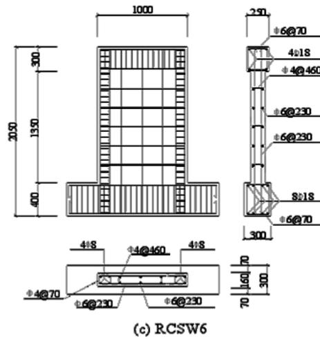
Figure 1. Reinforcement of test piece.
