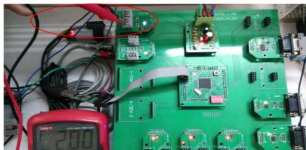
Figure 9. DAC0 analog output measurement figure.
