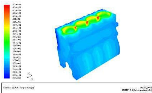
(1) Coupling bulk temperature field of the original mode.
