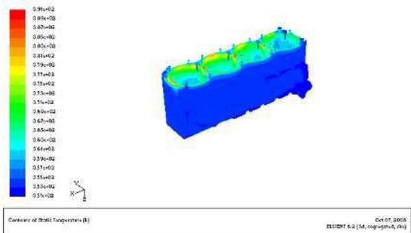
(4) Temperature field of outer wall of the first project.
