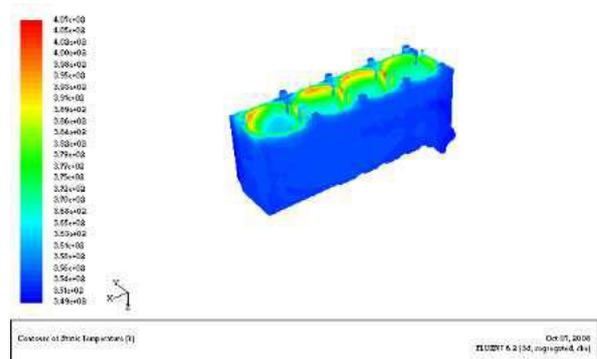
(2) Temperature field of outer wall of the original model.
