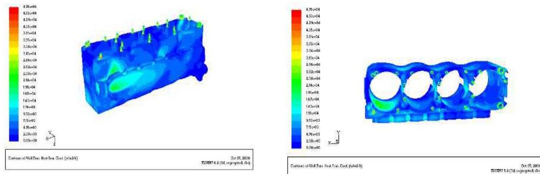
(2) Heat-transfer coefficient distribution of the first improved project's coolant jacket surfaces.
