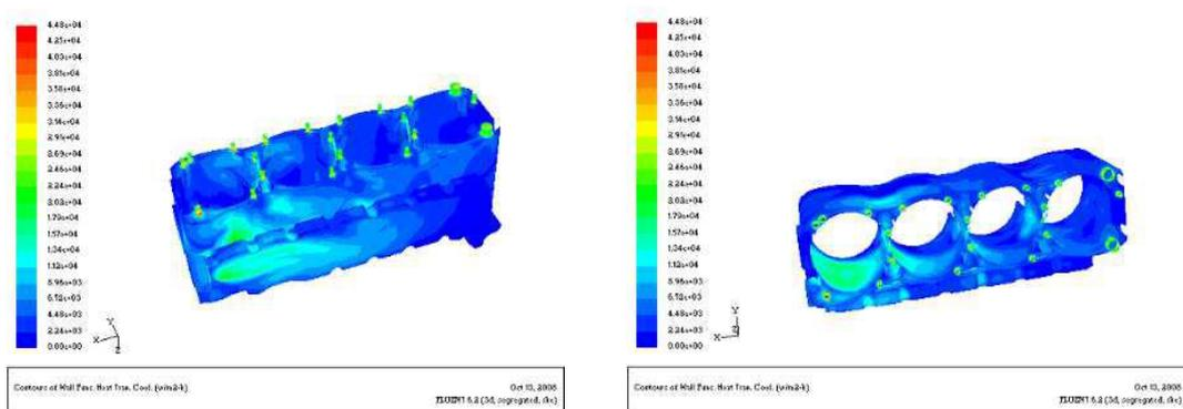
(3) Heat-transfer coefficient distribution of the second improved project's coolant jacket surfaces.
