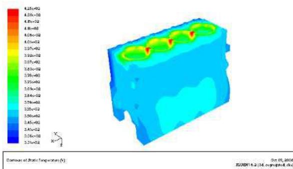
(3) Coupling bulk temperature field of the first project.
