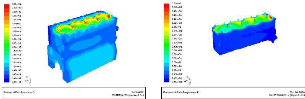
(5) Coupling bulk temperature field of the second project. (6) Temperature field of outer wall of the second project.
