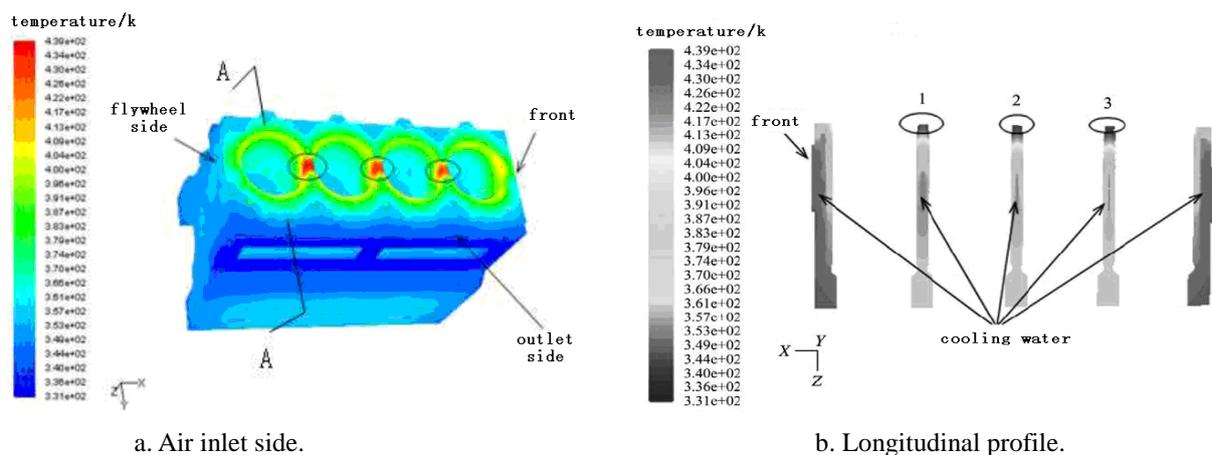
Note: 1, 2, 3 -- representing junction between the first cylinder to the fourth cylinder.
