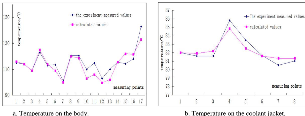
Figure 2. Comparison of temperature between calculation and test in system model.
