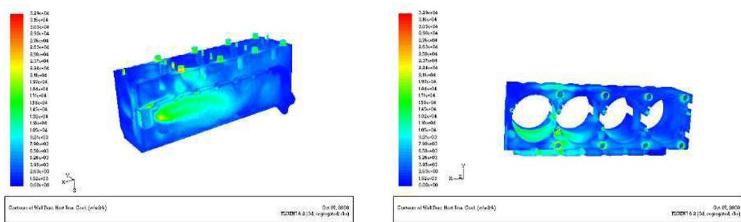
(1) Heat-transfer coefficient distribution of the original model's coolant jacket surfaces.
