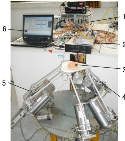
**Figure 2.** Prototype of six pyramid parallel mechanism.
