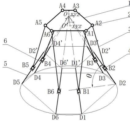
Figure 1. Sketch map of six-pyramid parallel mechanism.
