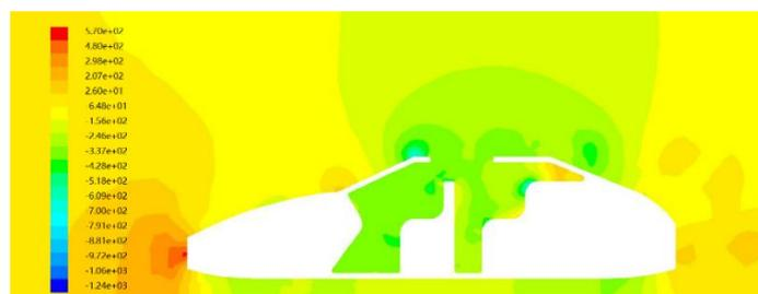
**Figure 17.** Pressure cloud chart of 'condition 4' in the improved car.
