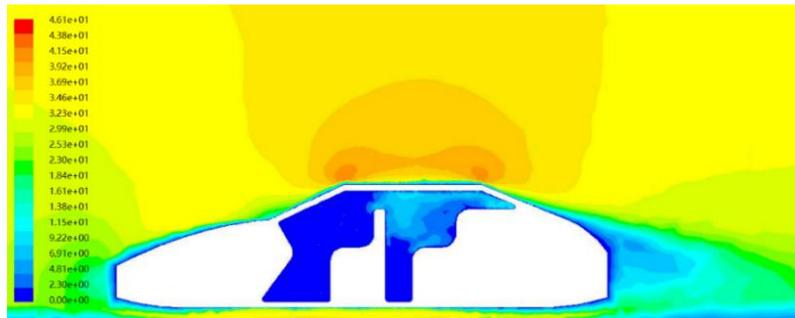
Figure 12. Velocity cloud chart of 'condition 3' in the car.
