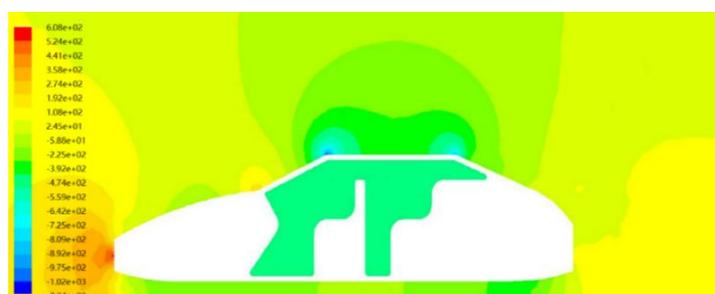
Figure 4. Pressure cloud chart of 'condition 1' in the car.
