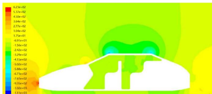
Figure 10. Pressure cloud chart of 'condition 3' in the car.
