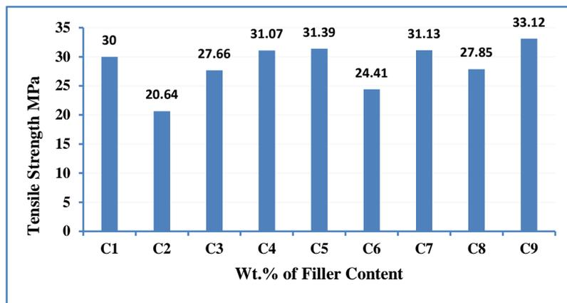
**Figure 4.** The influence of various composition of composite on tensile strength
