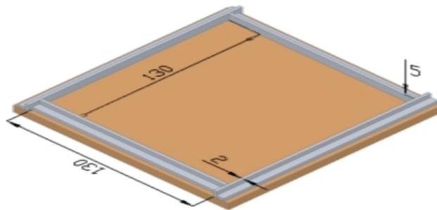
Figure 1. Dimensions and Shape of mould
