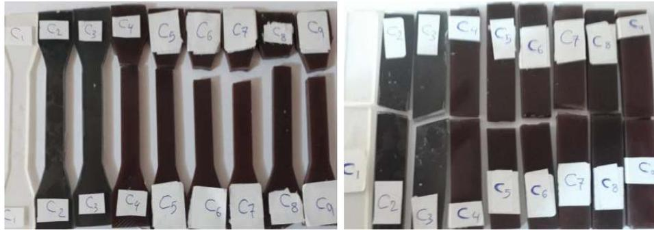
a) Specimens after tensile test      b) Specimens after flextural test
