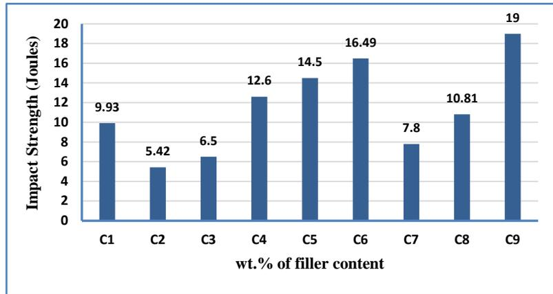
Figure 7. The influence of various composition of composite on impact strength property
