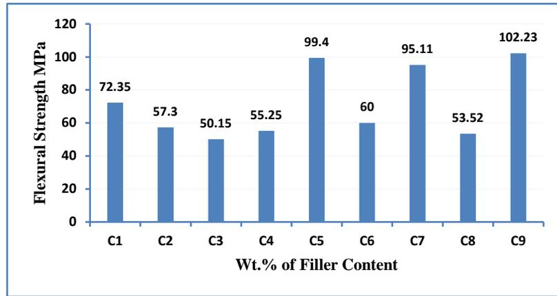
**Figure 5.** The influence of various composition of composite on flexural strength property
