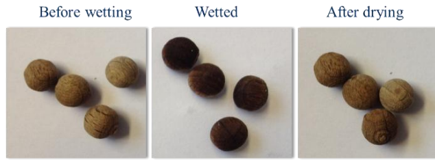
Figure 2. Wood particles before soaking, after soaking and after superheated steam drying.
