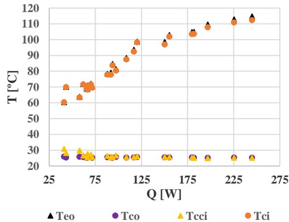
**Figure 7.** Temperatures at different locations vs heat load using water as the working fluid, using the new design evaporator
