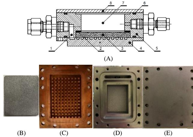
**Figure 4.** (A) Evaporator structure: vapor collector (1), silicone gasket (2), SS wick (3), copper base (4), SS body (5), O-ring (6), compensation chamber (7), SS lid (8); (B) Stainless steel sintered wick; (C) copper base of evaporator; (D) SS body; (E) SS lid
