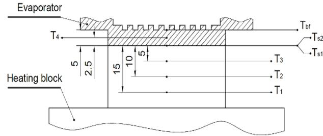
**Figure 3.** Temperature measurement inside heating block
