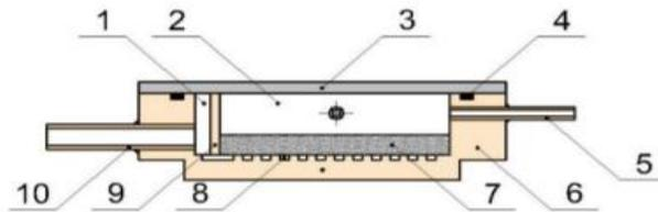
**Figure 1.** Schematic diagram of the previous evaporator 1: vapor collector; 2: compensation chamber; 3: poly carbonate lid; 4: O-ring; 5: charging pipe; 6: copper evaporator body; 7: wick; 8: vapor grooves; 9: copper plate; 10: vapor pipe.
