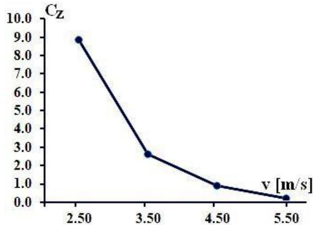
Figure 11. Resistant coefficient of explorer submarine when it rises.
