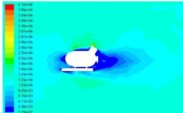
**Figure 4.** Contour of dynamic pressure of the explorer submarine with speed of 4.88 m/s, forward at 10 m depth.
