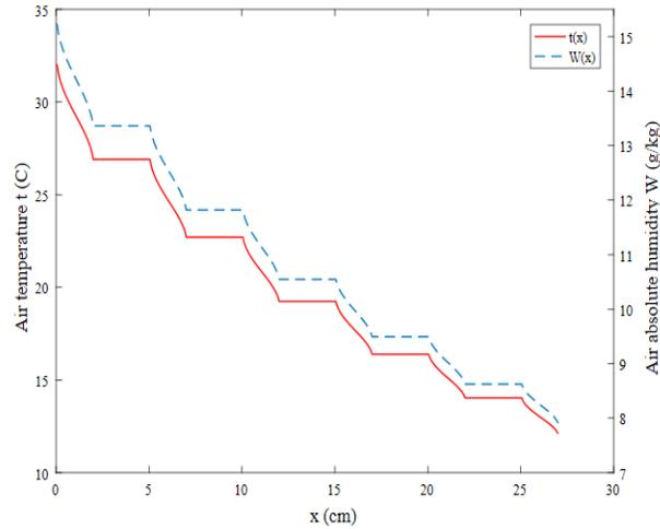
**Figure 4.** Variation of absolute humidity and temperature of moist air along the coil for the 1<sup>st</sup> case.
