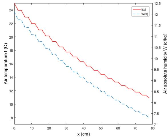
**Figure 5.** Variation of absolute humidity and temperature of moist air along the coil for the 2<sup>nd</sup> case.
