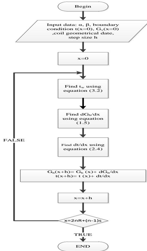
Figure 3. Flowchart of the simulation program
