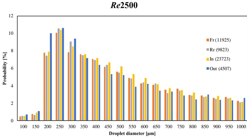
(a) The droplet diameter distribution at  $Re=2500$
