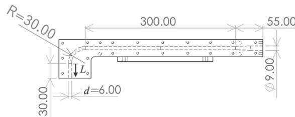
**Figure 1.** The size of nozzle for visualization experiment
