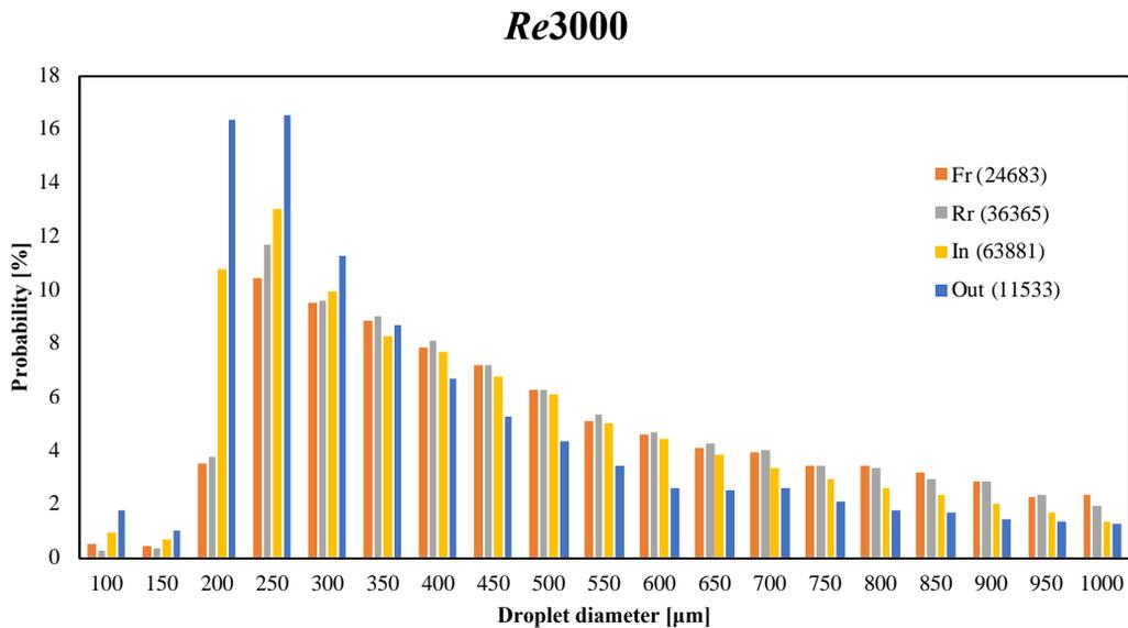
(b) The droplet diameter distribution at  $Re=3000$
