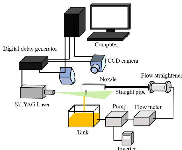
**Figure 4.** Experimental apparatus for stereo PIV experiment
