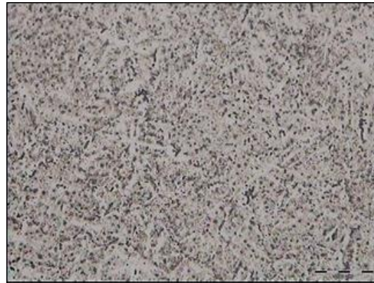
Figure 6. Optical microstructure in WZ of as-weld.
