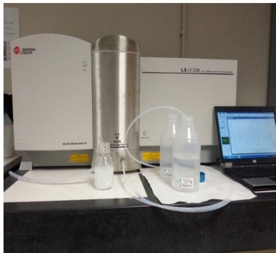
Figure 2. Laser diffraction particle size analyzer (LS 13 310)
