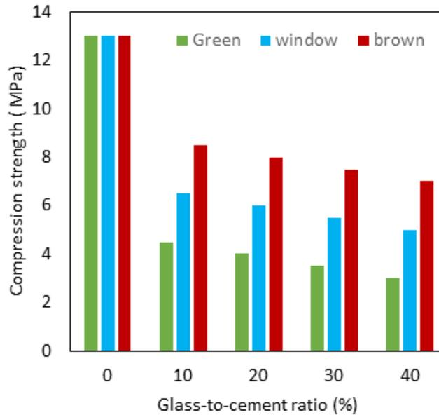
**Figure 8.** Compression of cement mortars after dip-coating with polyurethane polymer
