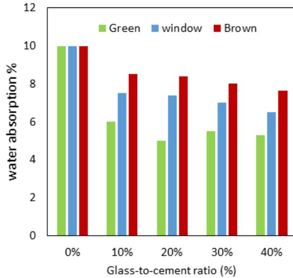
**Figure 4.** The water absorption of the cement mortars at different glass to cement ratios after dip-coating with polyurethane polymer
