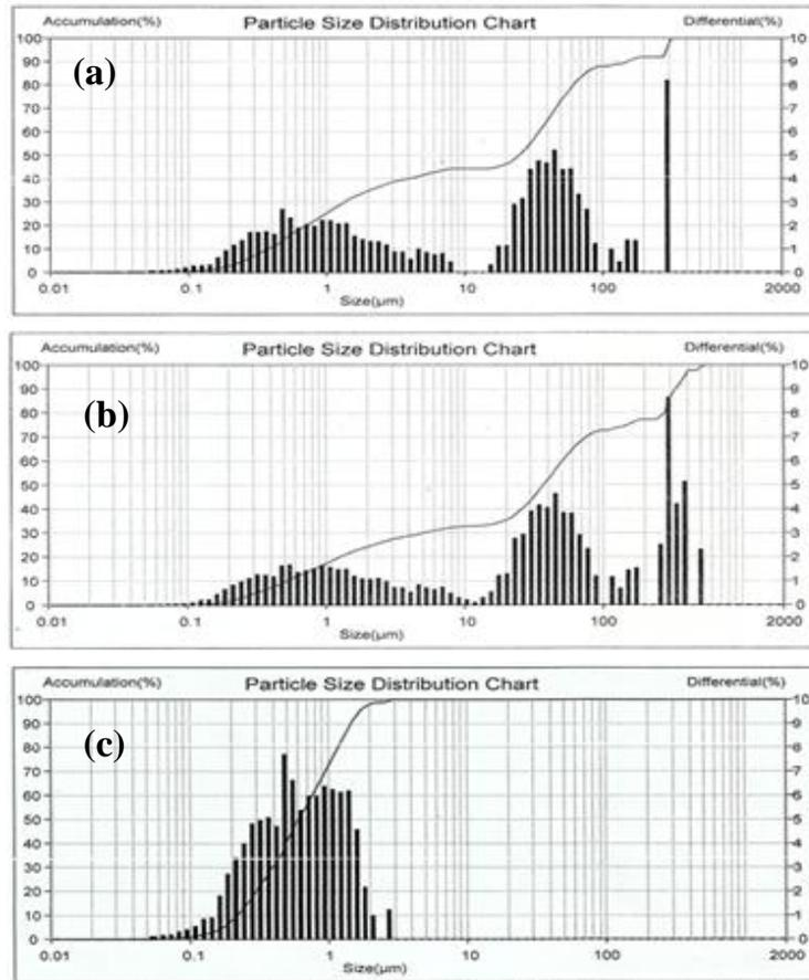
**Figure 1.** The particle size distributions of the glass powders. (a) Window sheet glass powder (b) Green-colored glass powder (c) brown-colored glass powder.
