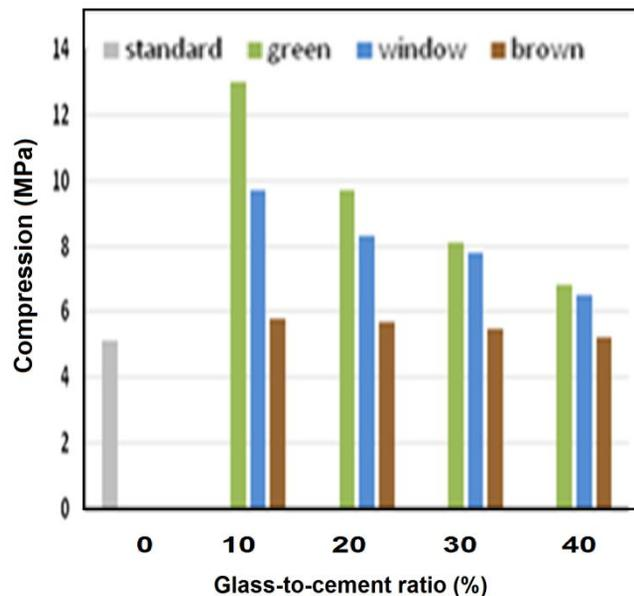
**Figure 7.** Compression of cement mortars before dip-coating with polyurethane polymer
