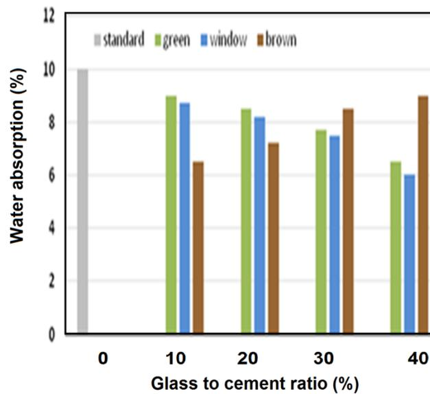
**Figure 3.** The water absorption of the cement mortars at different glass to cement ratios before dip-coating with polyurethane polymer
