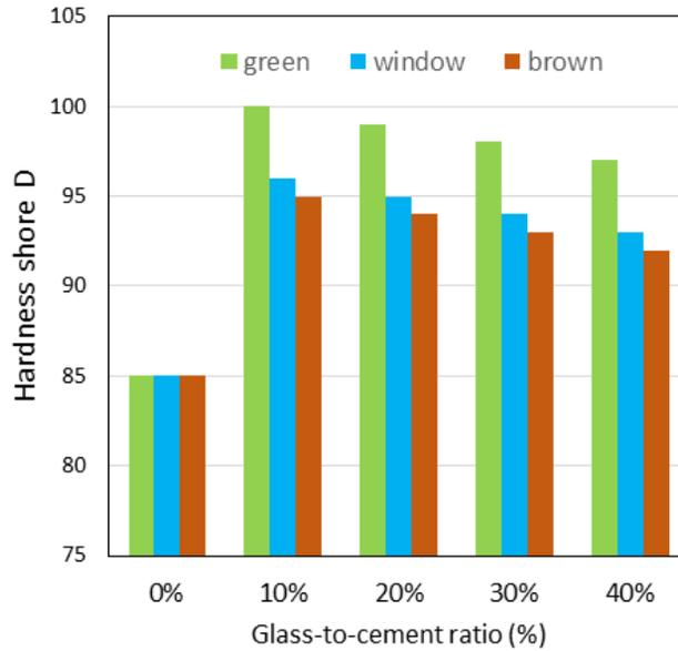
**Figure 6.** The hardness of cement mortars after dip-coating with polyurethane polymer
