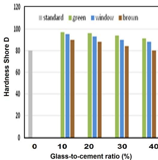
**Figure 5.** The hardness of cement mortars before dip-coating with polyurethane polymer
