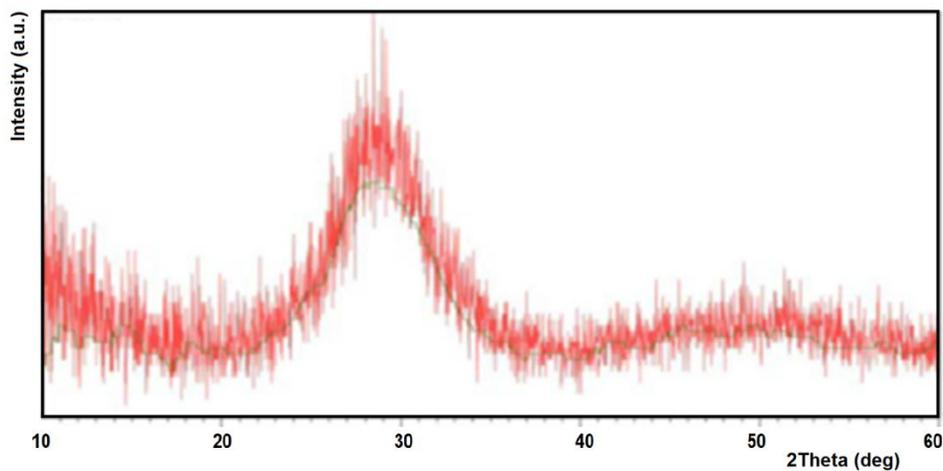
**Figure 2.** The XRD pattern of glass powders. All glass powders exhibited identical features to those measured
