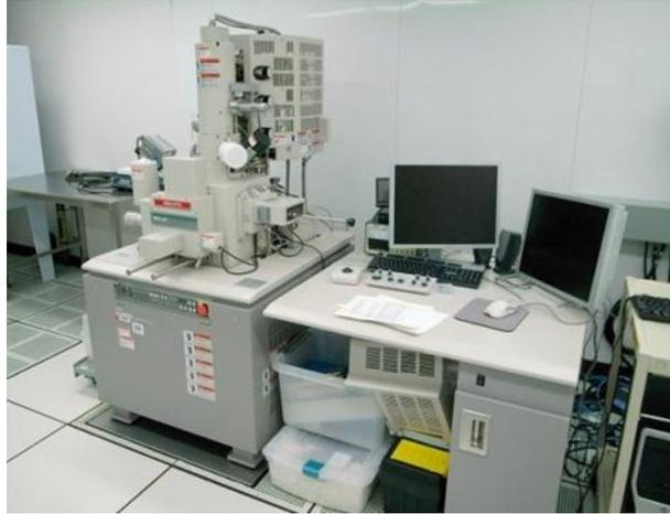
**Figure 6.** Scanning electron microscope FESEM Jeol 7600
