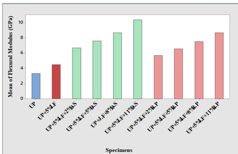
Figure 6. Results flexural modulus of all specimens
