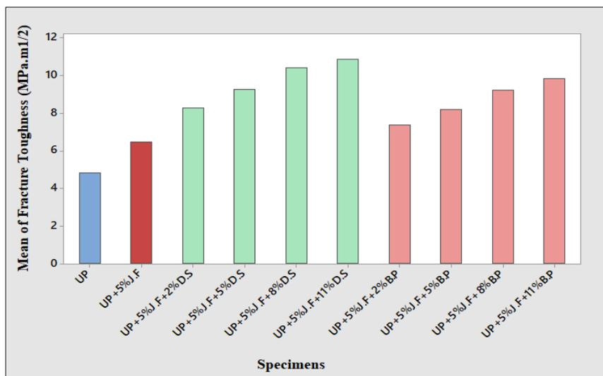
Figure 8. Results fracture toughness of all specimens
