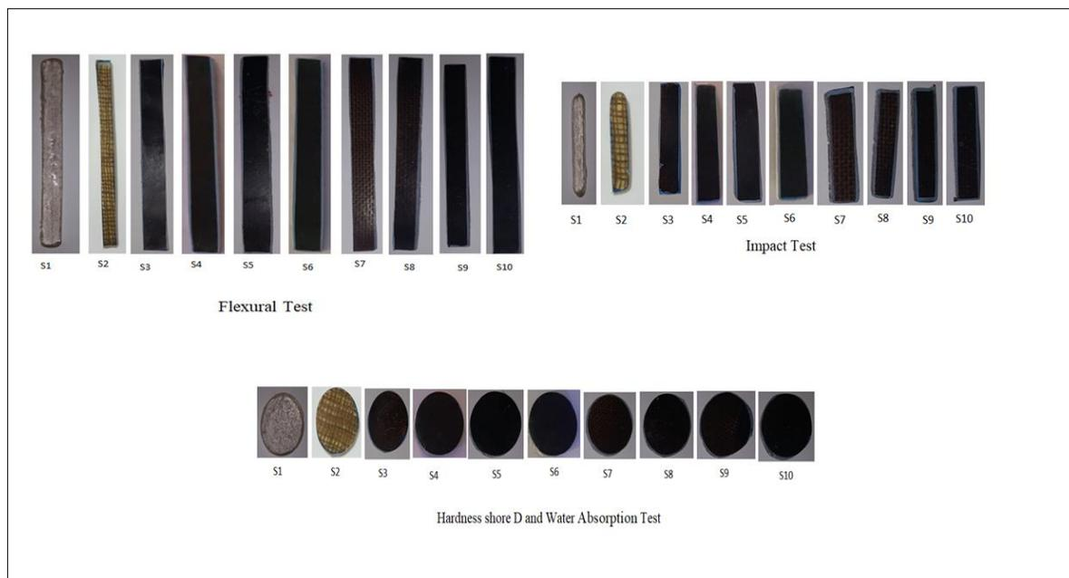
Figure 4. Specimens for flexural, impact and hardness shore D and water absorption
