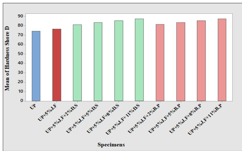
Figure 9. Results hardness shore D of all specimens
