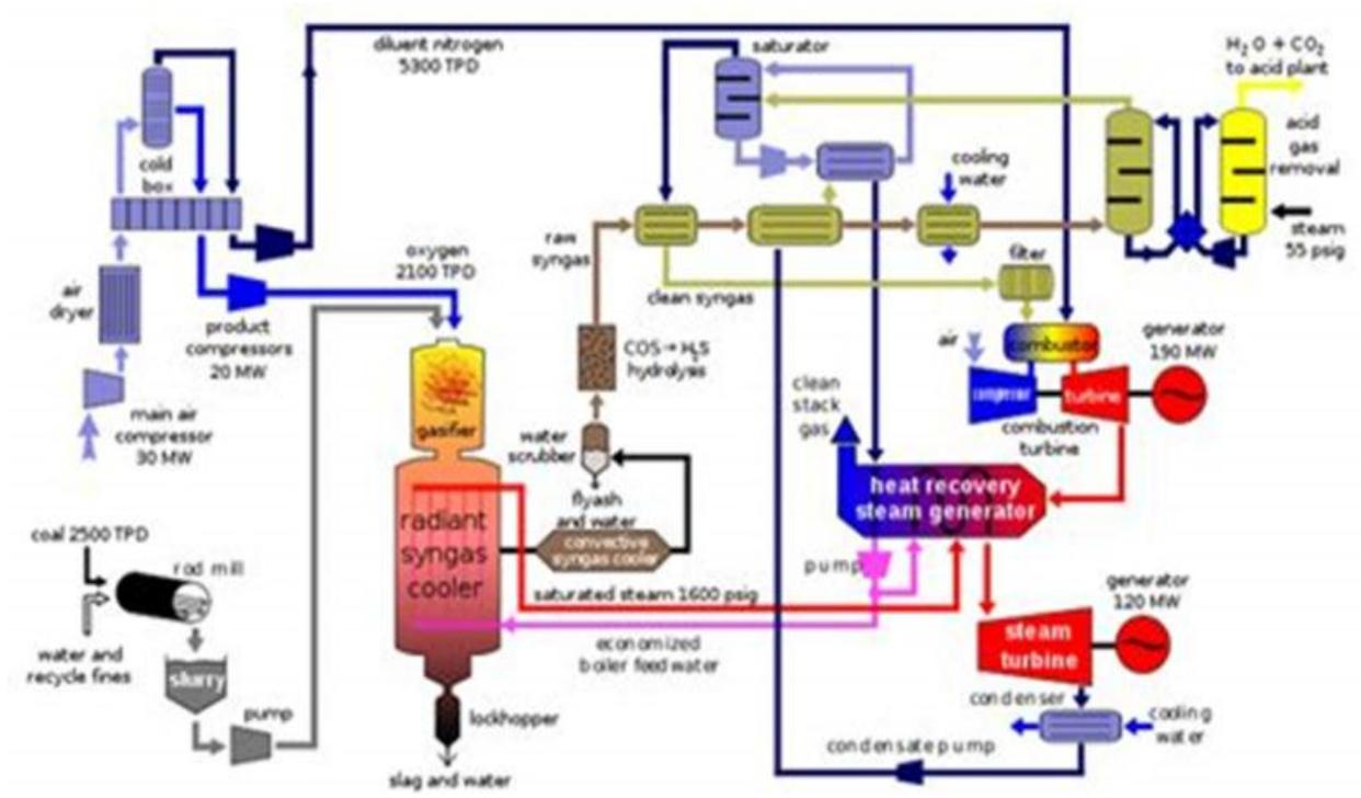
Figure 2. Process flow diagram in combined cycle power plant
