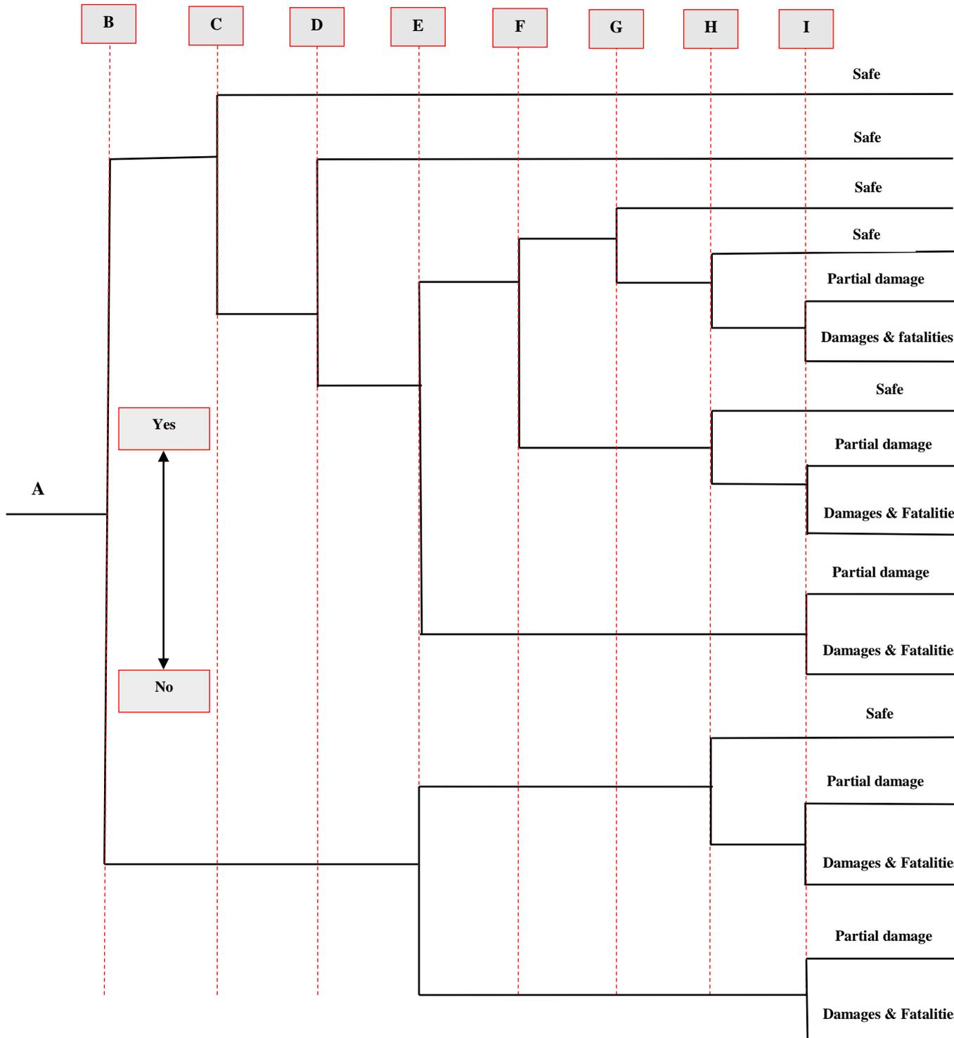
**Figure 4.** Typical event tree for an initiating event that represents water level fall below design limit inside steam boiler
