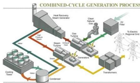
Figure 1. Combined cycle power plant
