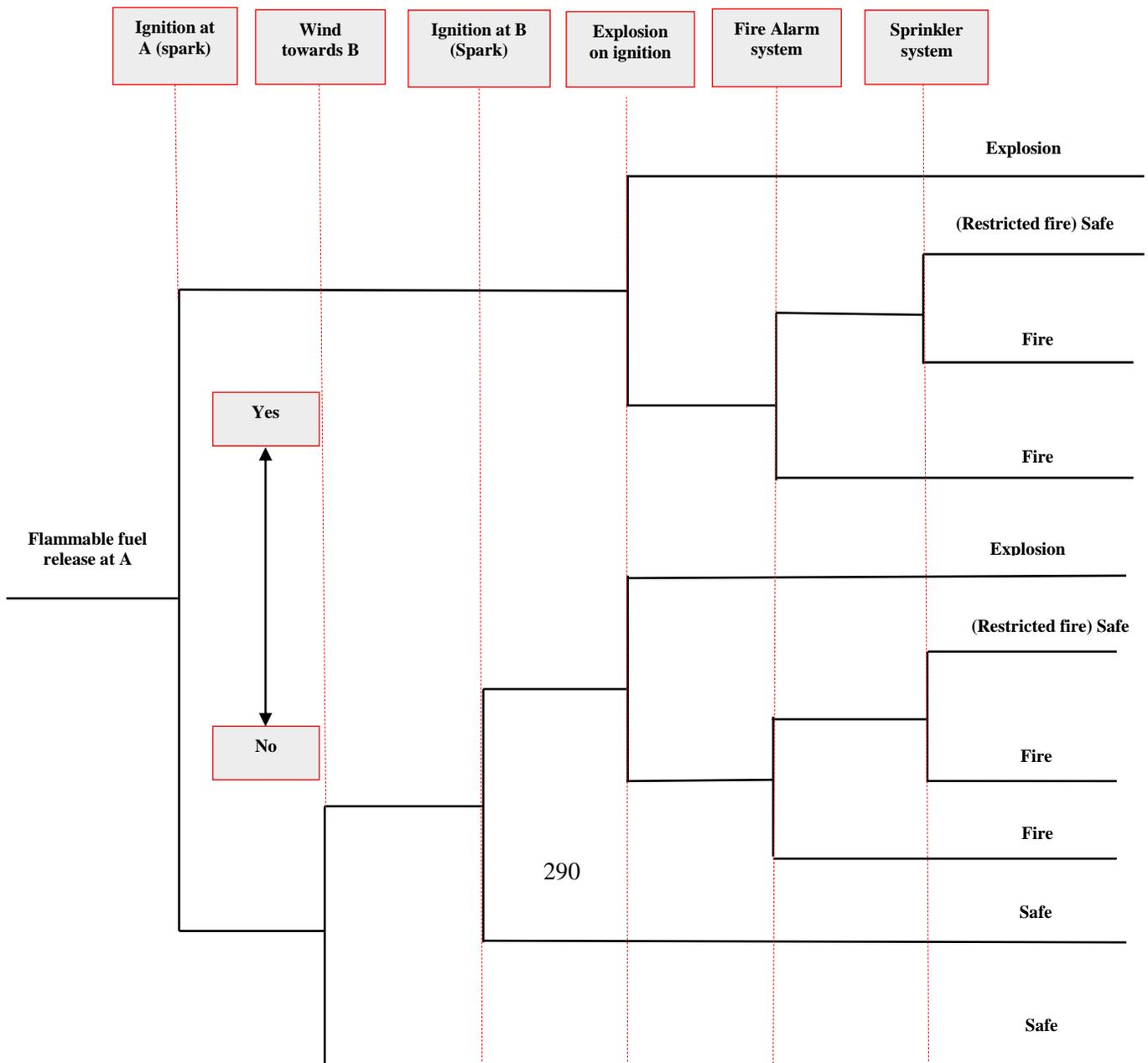
**Figure 3.** Typical event tree for flammable fuel spillage initiating event
