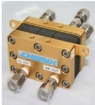
Figure 1. Photograph of PEFC short stack
