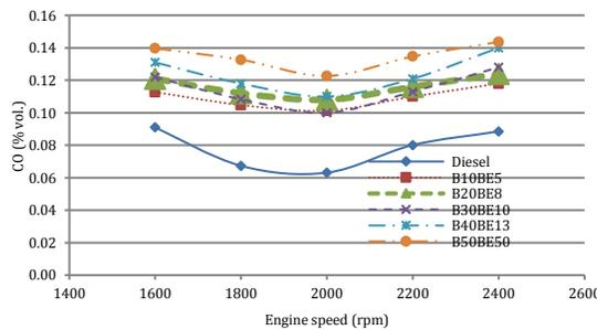
**Figure 8.** Variation of the CO emissions for biodiesel-bioethanol-diesel blends at full load and various engine speeds
