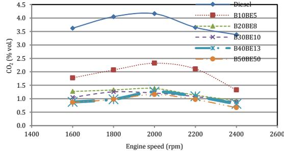
**Figure 9.** Variation of the CO<sub>2</sub> emissions for biodiesel-bioethanol-diesel blends at full load and various engine speeds
