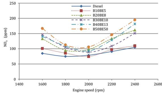
**Figure 7.** Variation of the NO<sub>x</sub> emissions for biodiesel-bioethanol-diesel blends at full load and various engine speeds
