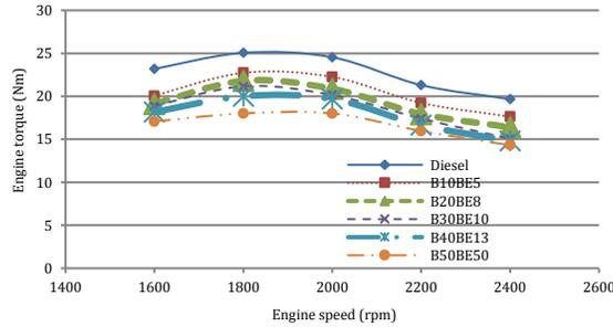
**Figure 3.** Variation of the engine torque for biodiesel-bioethanol-diesel blends at full load and various engine speeds
