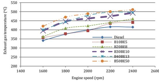
**Figure 5.** Variation of the exhaust gas temperature for biodiesel-bioethanol-diesel blends at full load and various engine speeds
