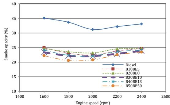
**Figure 10.** Variation of the smoke opacity for biodiesel-bioethanol-diesel blends at full load and various engine speeds
