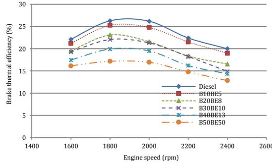
**Figure 6.** Variation of the brake thermal efficiency for biodiesel-bioethanol-diesel blends at full load and various engine speeds
