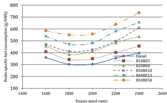
**Figure 2.** Variation of the brake specific fuel consumption for biodiesel-bioethanol-diesel blends at full load and various engine speeds
