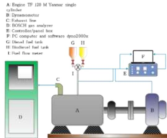
**Figure 1.** Schematic layout of the single-cylinder direct injection diesel engine set-up
