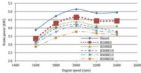
**Figure 4.** Variation of the brake power for biodiesel-bioethanol-diesel blends at full load and various engine speeds
