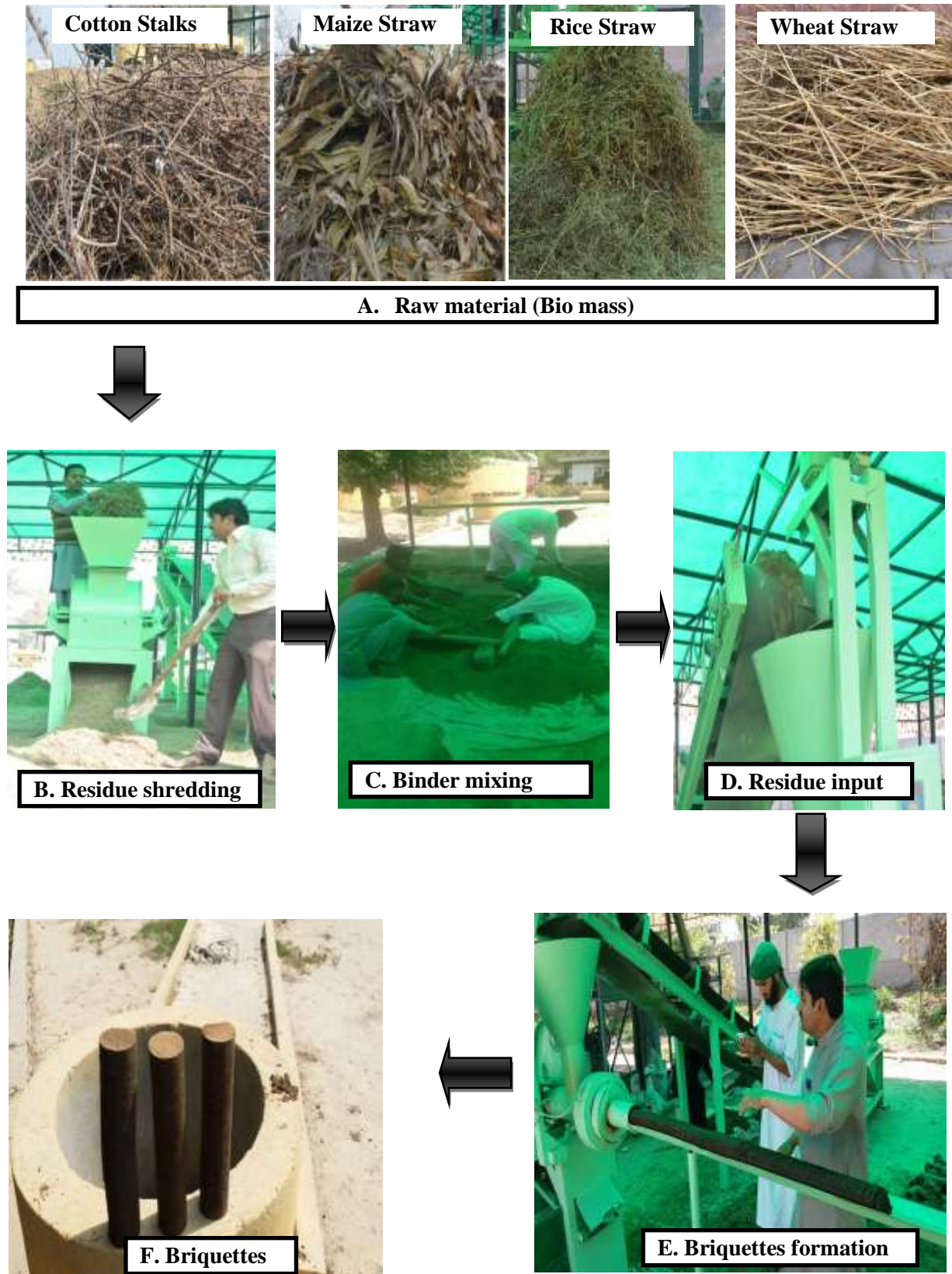
Figure 7. Flow diagram of briquette formation from raw materials content
