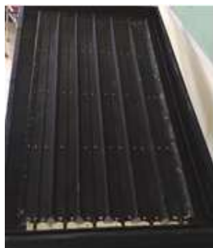
Figure 3. V-shaped absorber plate with PCM storage
