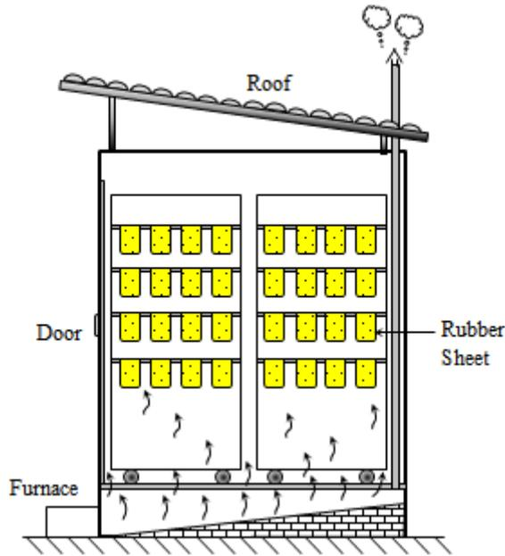
Figure 1. Direct method of air heating for conventional rubber drying room.
