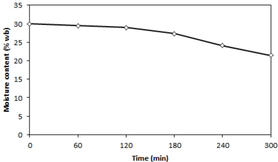
**Figure 9.** Variation of moisture content in rubber sheet with time
