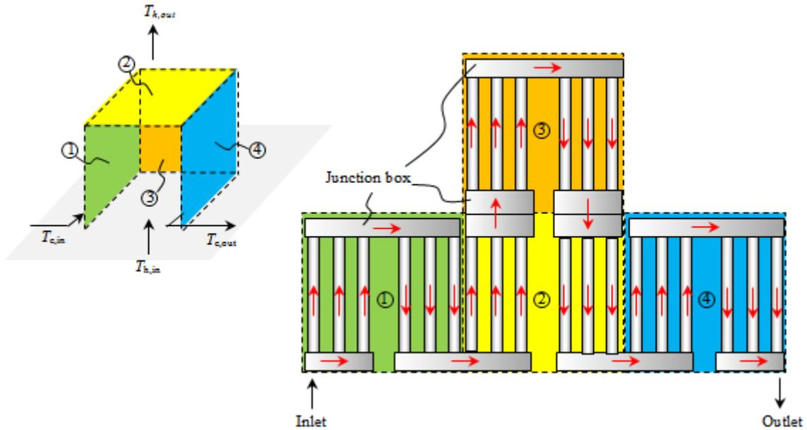
**Figure 3.** Schematic diagram of the air flow path in multi-tube passes heat exchanger.
