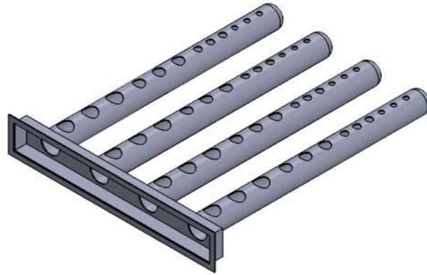
**Figure 5.** Perforate branch pipes for uniform distribution air flow in drying chamber.
