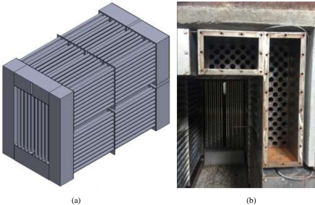
**Figure 4.** (a) Back side view of heat exchanger model, (b) Installation of heat exchanger in the combustion chamber of biomass furnace.
