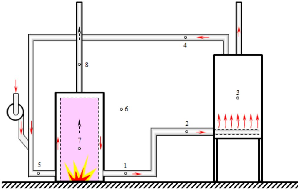
**Figure 6.** Positions of temperature measurement in drying system
