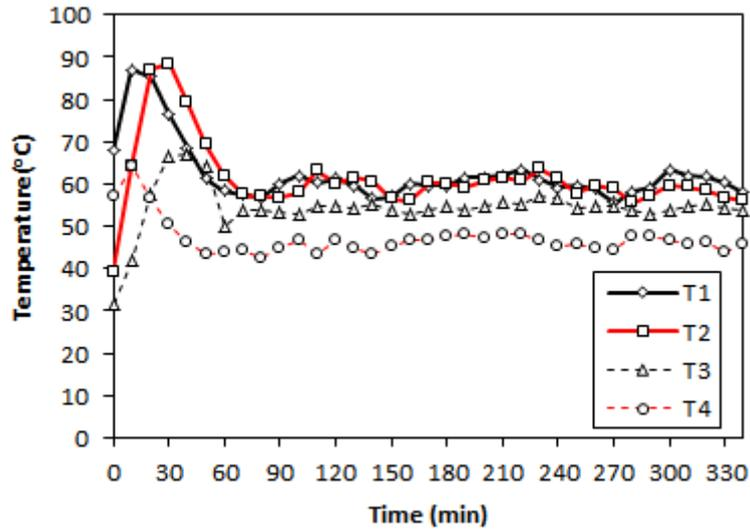
**Figure 7.** Variation of temperature with time at various positions when firewood feed rate was 3 kg/h in the first hour and 1 kg/h in the subsequent hours.
