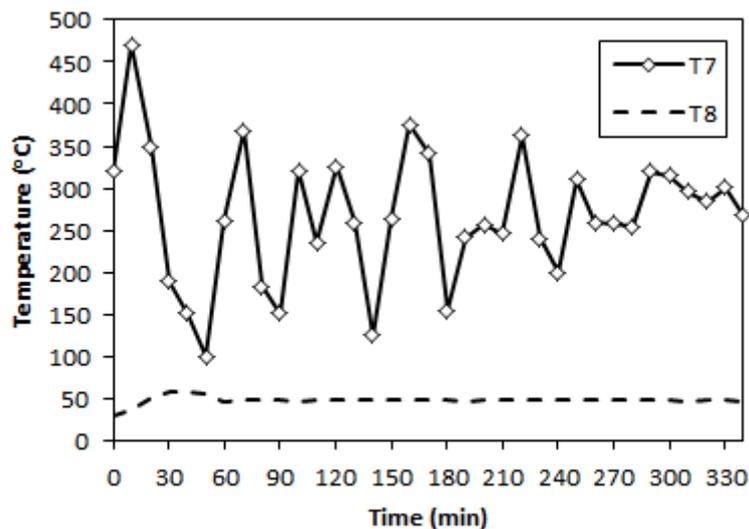
**Figure 8.** Variation of flue gas temperature with time
