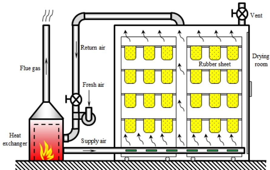
Figure 2. Indirect method of air heating for rubber drying room.
