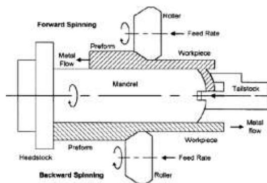
**Figure 1.** Forward Spinning process principle
