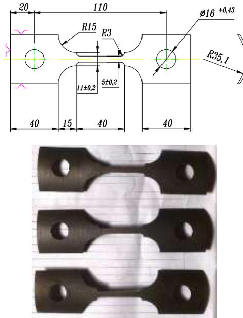
**Figure 12.** Tensile testing sample from spinning workpieces
