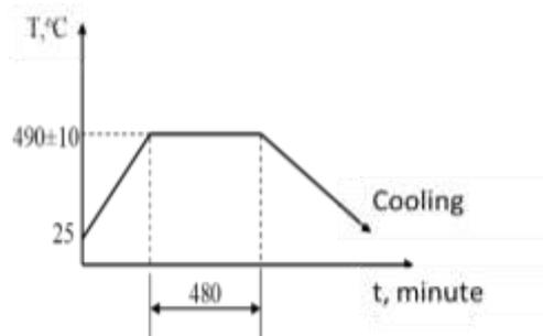
**Figure 8.** Heat treatment of workpiece
