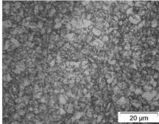
**Figure 9.** Microstructure of sample after step 1<sup>st</sup> spinning (2.1mm thickness), x 1000
