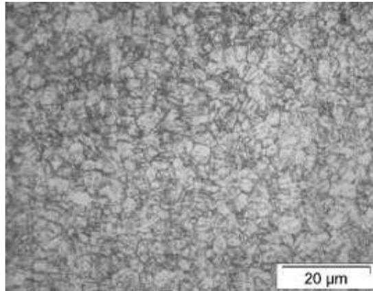
**Figure 10.** Microstructure of sample after step 2<sup>nd</sup> spinning (1.1mm thickness), x 1000
