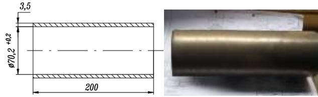
Figure 2. Spinning workpiece dimensions
