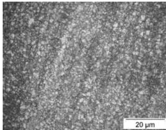
**Figure 11.** Microstructure of sample after step 3<sup>rd</sup> spinning (0.48 mm thickness), x 1000
