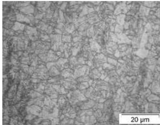
Figure 3. Workpiece microstructure before tubular formation, x1000
