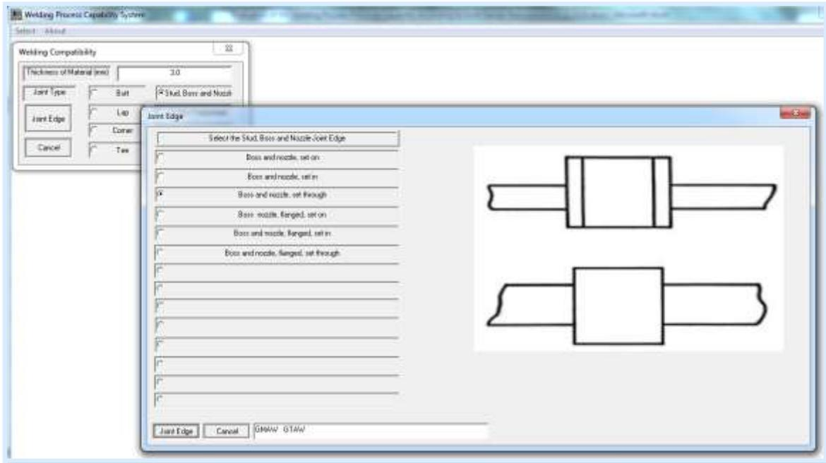
Figure 10. Welding compatibility form showing the joint edges types that corresponding to (Stud, Boss And Nozzle) joint
