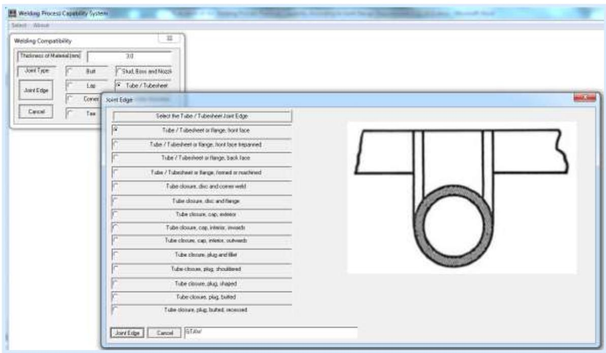
Figure 11. Welding compatibility form showing the joint edges types that corresponding to (Tube / Tube-Sheet) joint
