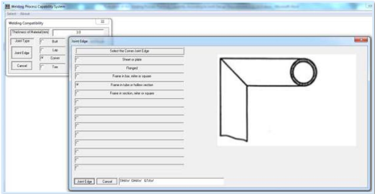
Figure 8. Welding compatibility form showing the joint edges types that corresponding to (Corner) joint
