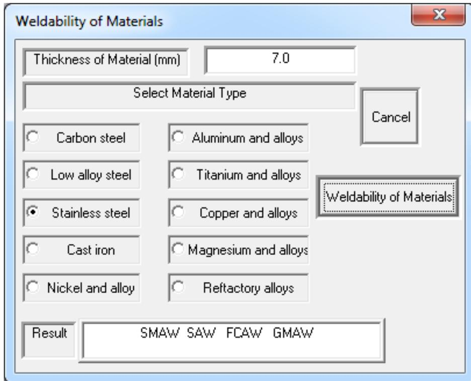
Figure 4. Weldability of material form
