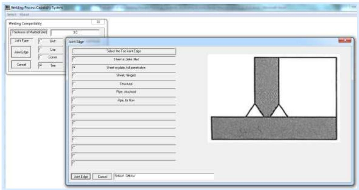
Figure 9. Welding compatibility form showing the joint edges types that corresponding to (Tee) joint
