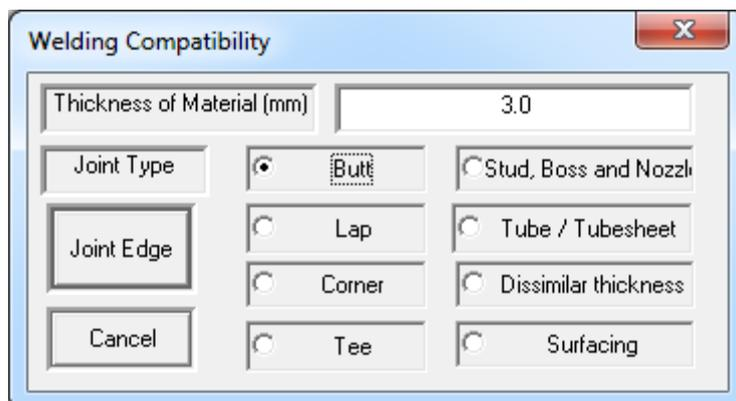
Figure 5. Welding compatibility form
