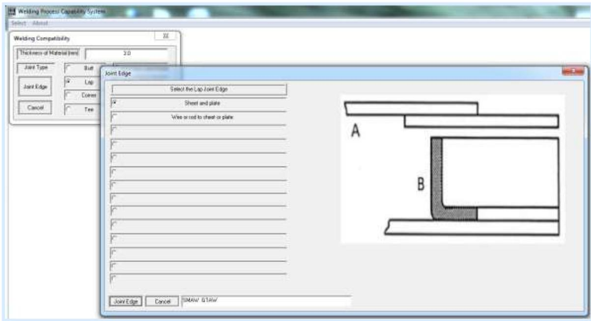
Figure 7. Welding compatibility form showing the joint edges types that corresponding to (Lap) joint
