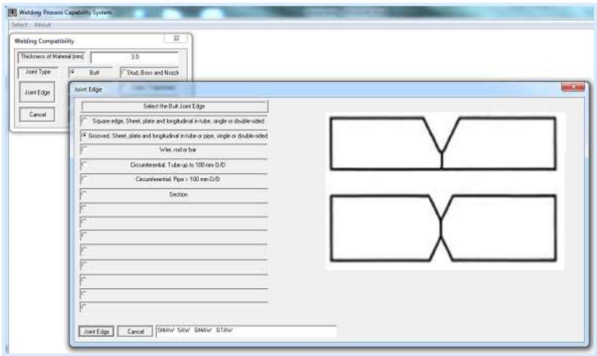
Figure 6. Welding compatibility form showing the joint edges types that corresponding to (Butt) joint
