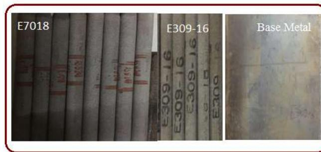
**Figure 1.** Shown the base metal and electrodes E7018 & E309-16
