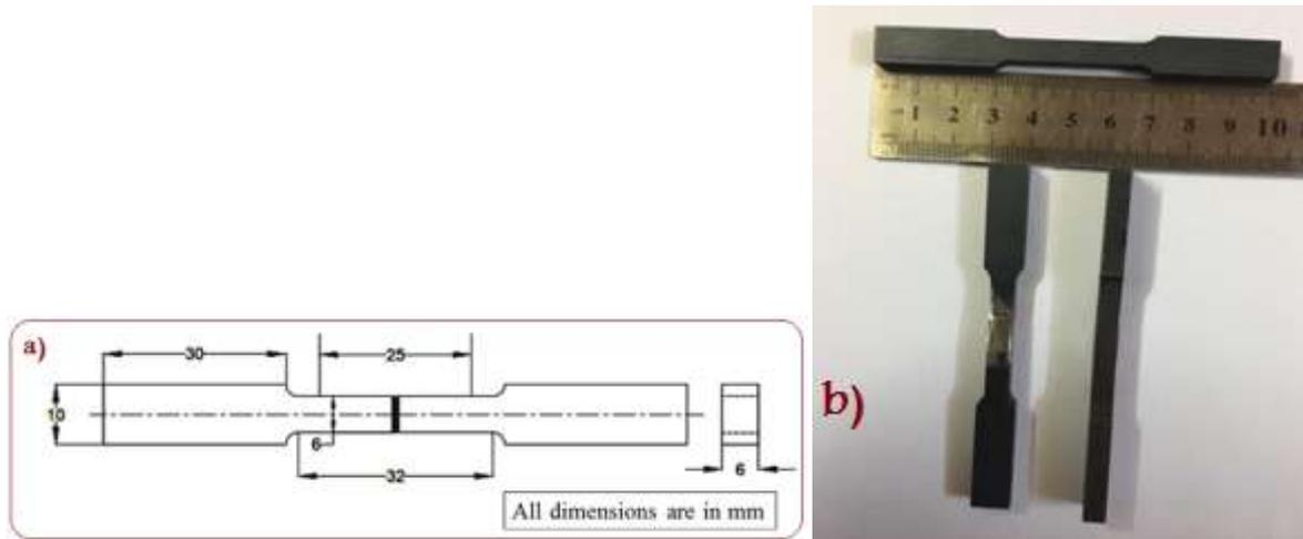
**Figure 3.** Shown tensile specimen: a) The standard dimensions of tensile testing specimen, b) Tensile specimen
