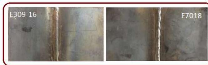
**Figure 2.** Shown base metal of carbon steel welded by E7018 & E309-16
