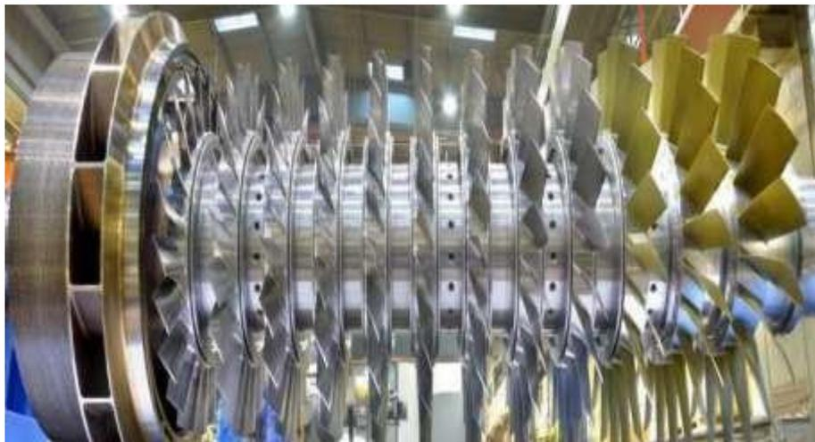
**Figure 1.** Axial flow compressor
