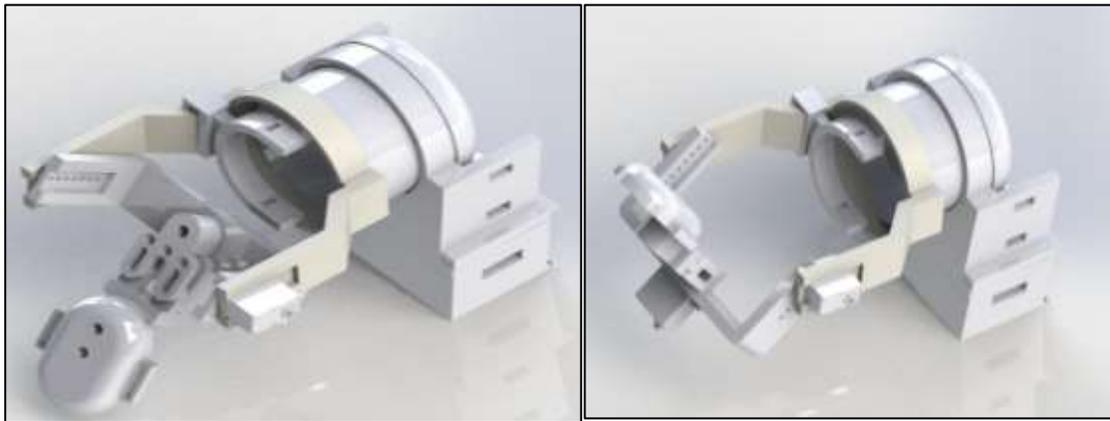
**Figure 13.** Flexion (above) and Extension (below) Movement of the Exoskeleton
