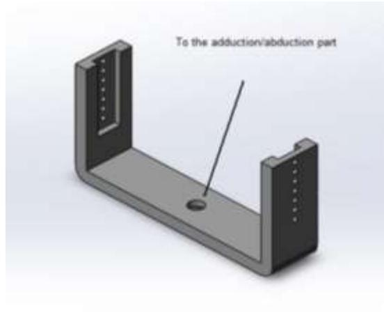
**Figure 3.** CAD Model of the Flexion /Extension Part.
