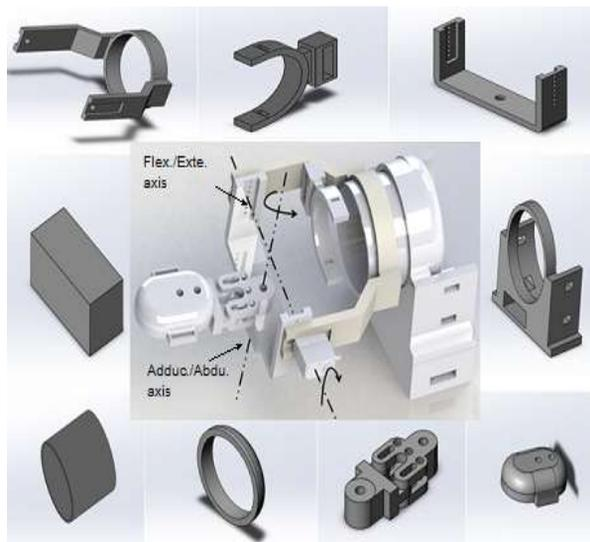
**Figure 6.** Parts Constructing the Exoskeleton and their Assembly
