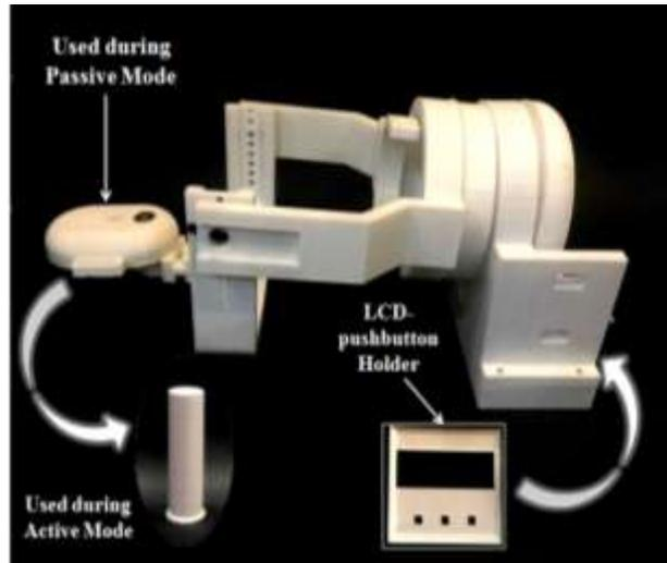
Figure 9. Exoskeleton Assembly
