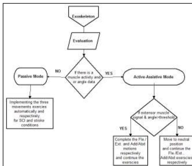
Figure 12. Schematic Diagram of the Exoskeleton Working
