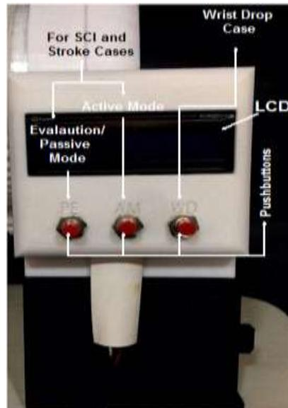
Figure 11. Assembly of LCD and pushbuttons with exoskeleton
