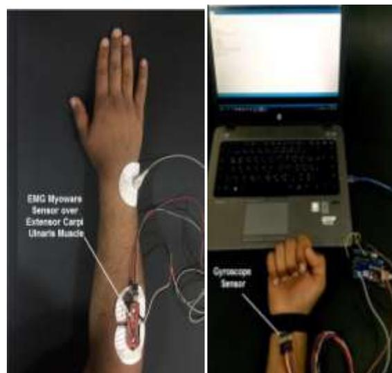
Figure 10. Muscle Activity and Angle Measurements
