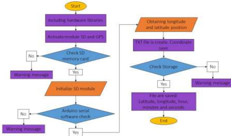
**Figure 14.** Arduino Algorithm Flowchart
