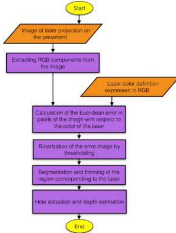
**Figure 5.** Image Processing Algorithm Flowchart.
