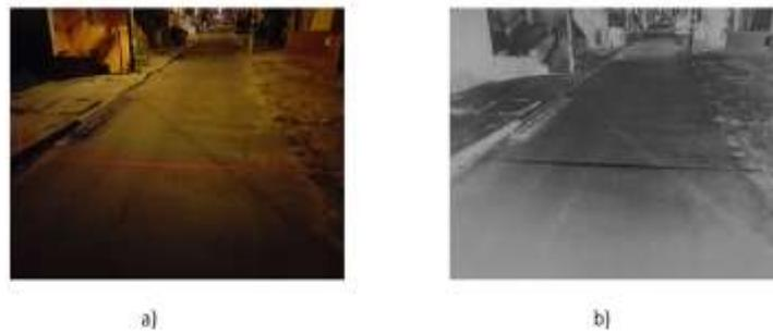
**Figure 6.** Laser's Image Projection on the Pavement **a)** original image **b)** image corresponding to the Euclidean error taking the laser's color as a reference
