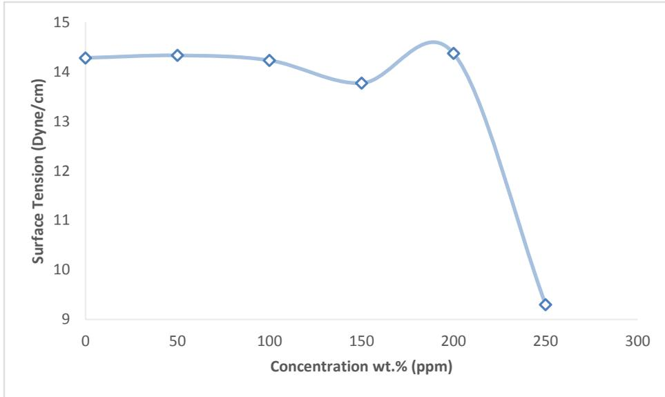
**Figure 13.** Surface tension of crude oil which includes different concentrations of PAA (0, 50, 100, 150, 200 and 250 ppm)
