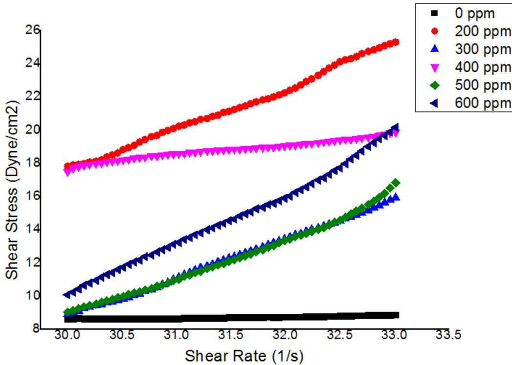
**Figure 10.** Shear stress – shear rate behavior of crude oil which includes different PEG concentrations (0, 200, 300, 400, 500 and 600 ppm)
