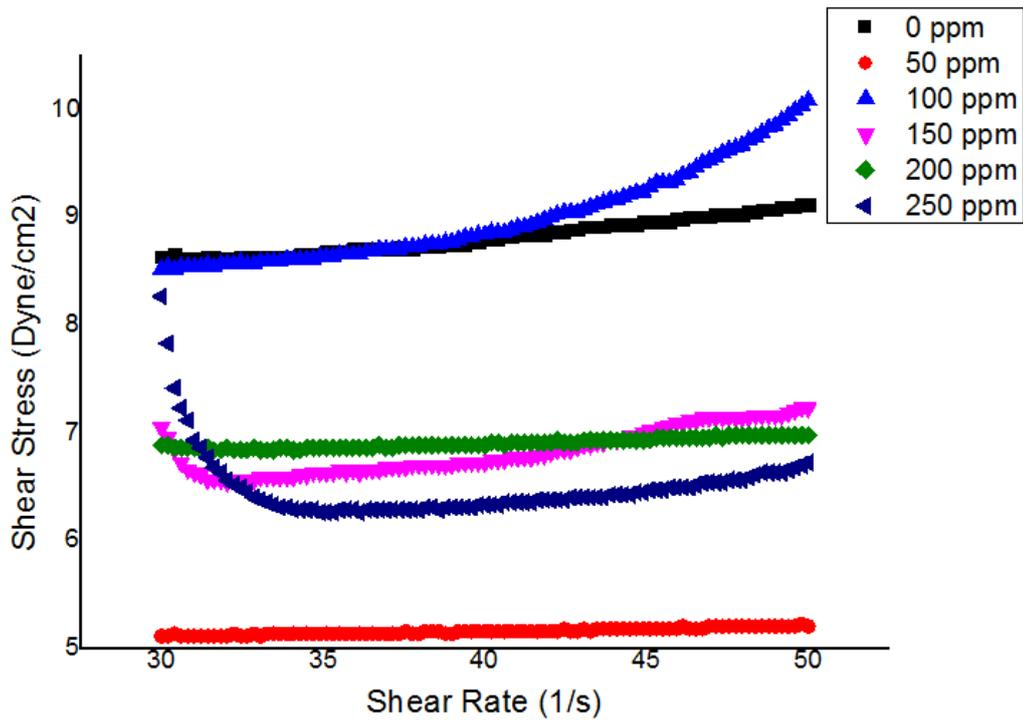
**Figure 7.** Shear stress – shear rate behavior of crude which having different PAA concentrations (0, 50, 100, 150, 200 and 250 ppm)
