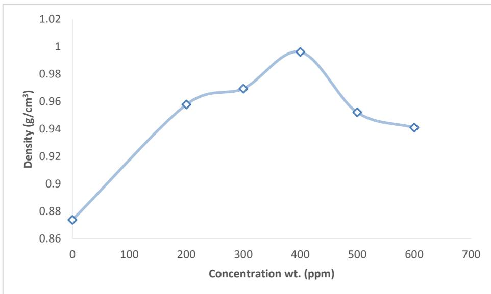
**Figure 12.** Density curve of crude oil which includes different PEG concentrations (0, 200, 300, 400, 500 and 600 ppm)
