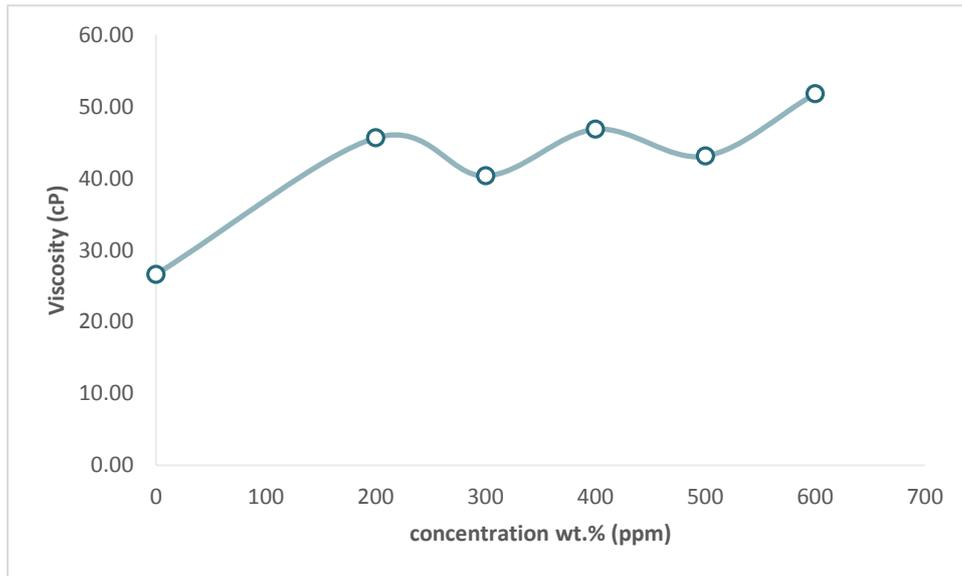
**Figure 8.** Viscosity behavior of crude oil which having different PEG concentrations (0, 200, 300, 400, 500 and 600 ppm)
