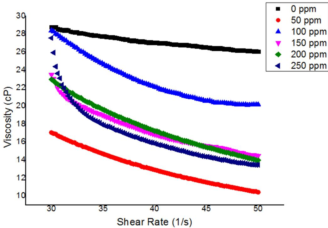
**Figure 6.** Viscosity-shear rate behavior of crude oil for different PAA concentrations (0, 50, 100, 150, 200 and 250 ppm)
