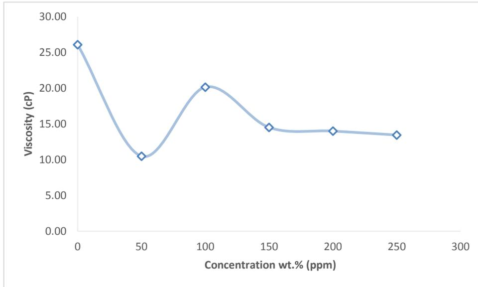
**Figure 5.** Viscosity behavior of crude oil as a function of PAA concentrations (0, 50, 100, 150, 200 and 250 ppm).
