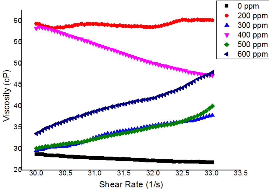
**Figure 9.** Viscosity-shear rate behavior of crude oil which includes different PEG concentrations (0, 200, 300, 400, 500 and 600 ppm)
