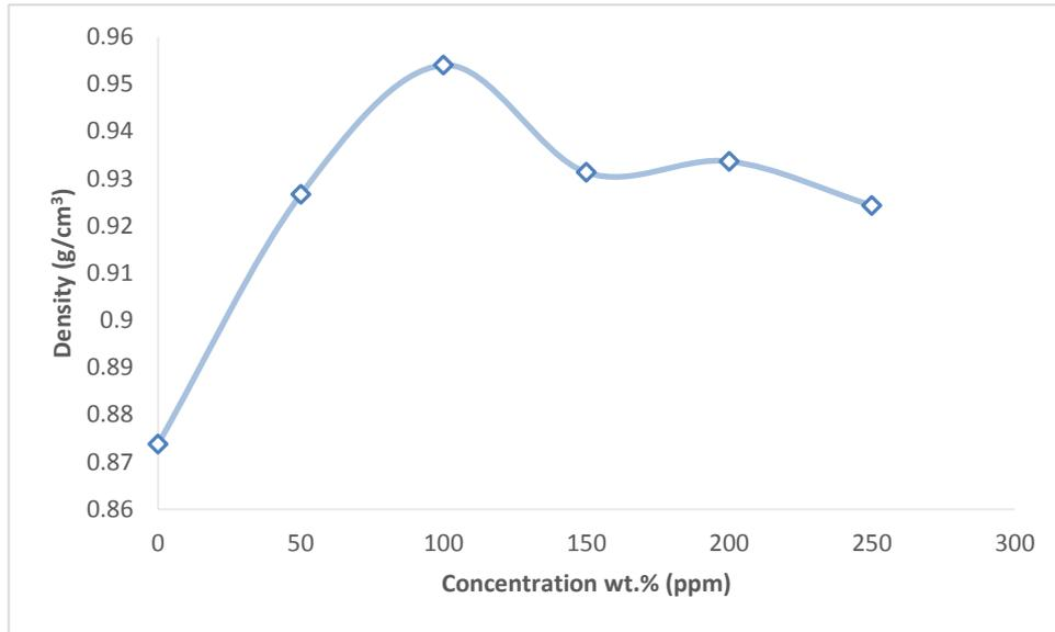
**Figure 11.** Density curve of crude oil which includes different PPA concentrations (0, 50, 100, 150, 200 and 250 ppm)
