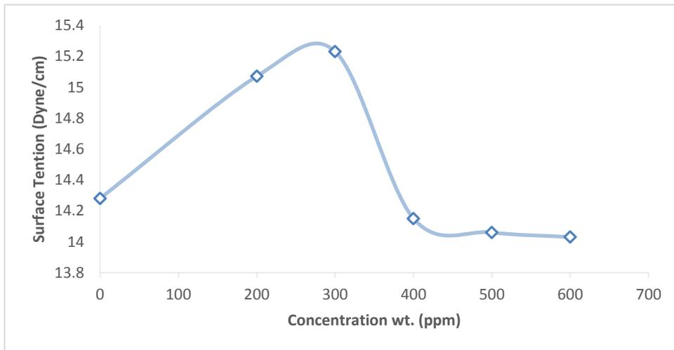
**Figure 14.** Surface tension of crude oil which includes different concentrations of PEG (0, 200, 300, 400, 500 and 600 ppm)
