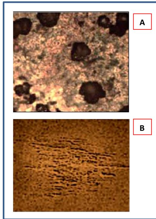
**Figure 8:** Surface metallography damage for; (a) untreated and (b) laser treated samples after corrosion in the 13% HCl solution.
