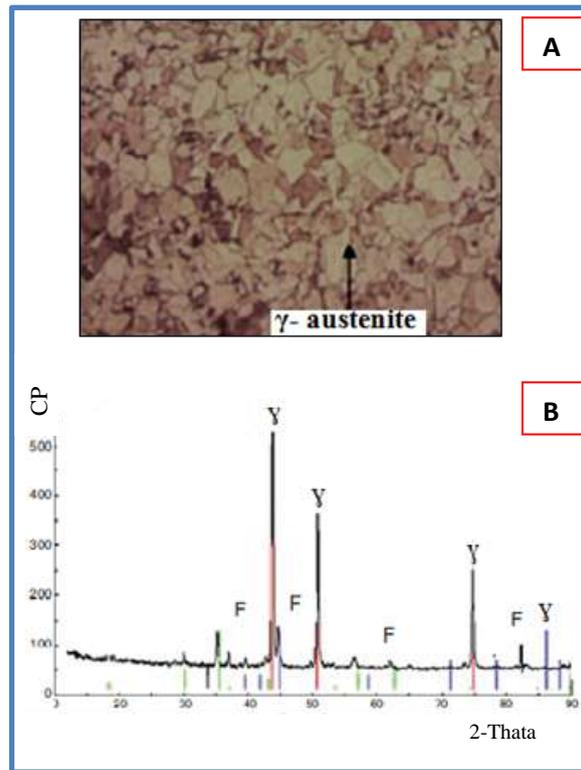
**Figure 4:** A - Microstructure of 304 stainless steel before laser at 200x and, B - XRD analyses after laser treatment.
