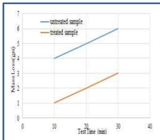
**Figure 9:** Wear test results before and after laser treatment of sample 304 stainless steel.
