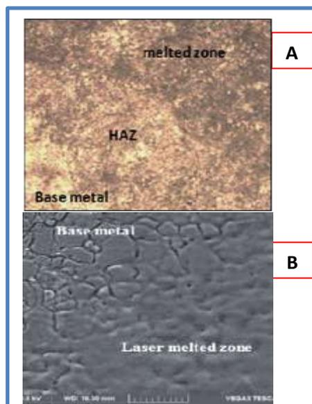
**Figure 5:** Optical micrograph (A) and; SEM images (B) for the laser treated sample, 100x.
