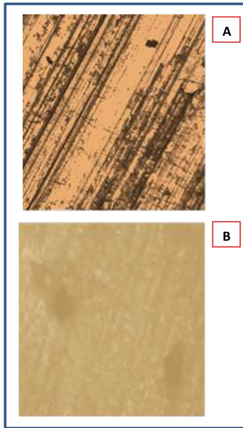
**Figure 10:** Micrographs of surface damages after wear test; A, before laser and B, after laser, 400x.
