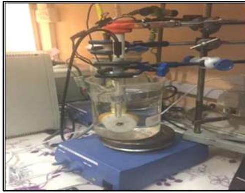
**Figure 2:** Electrochemical corrosion cell
