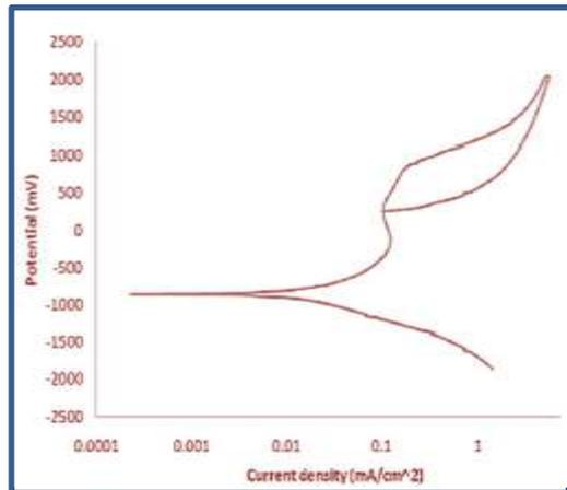
**Figure 6:** Polarization curves path for untreated sample AISI 304 stainless steel.
