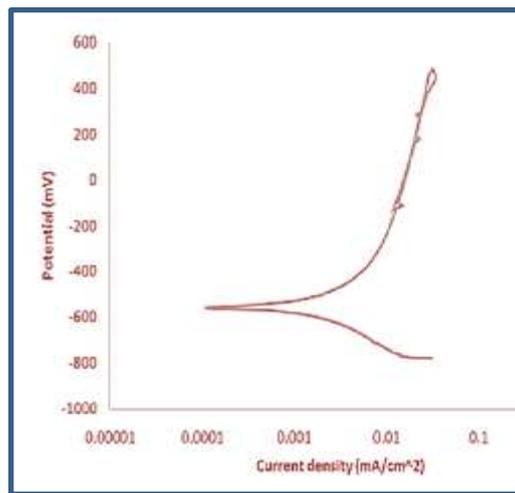
**Figure 7:** Polarization curves path for laser treated sample AISI 304 stainless steel.
