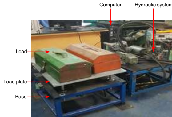
Figure 6. Photograph of the hydraulic vibration shaker
