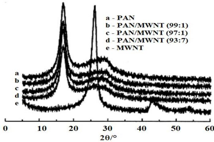
Figure 5. X-ray diffraction curves of fibers with different carbon tube contents and control samples
