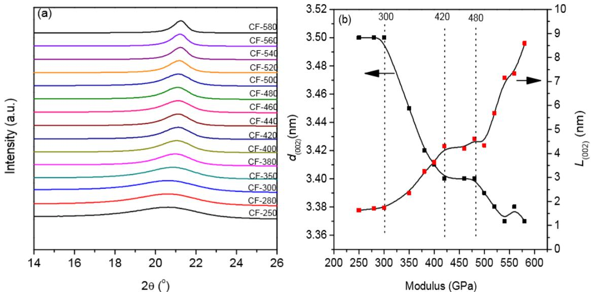
**Figure 7.** Carbon fiber crystallite structure parameters: (a) (002) plane wide-angle X-ray integral diagram (b) crystal plane spacing and grain size change with changes in carbon fiber modulus.
