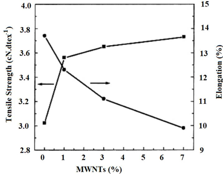
Figure 3. Mechanical properties of PAN / MWNT fibers
