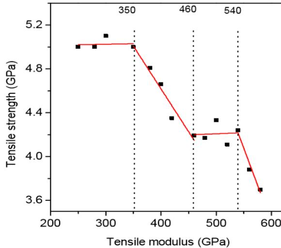
Figure 6. Tensile strength changes with tensile modulus
