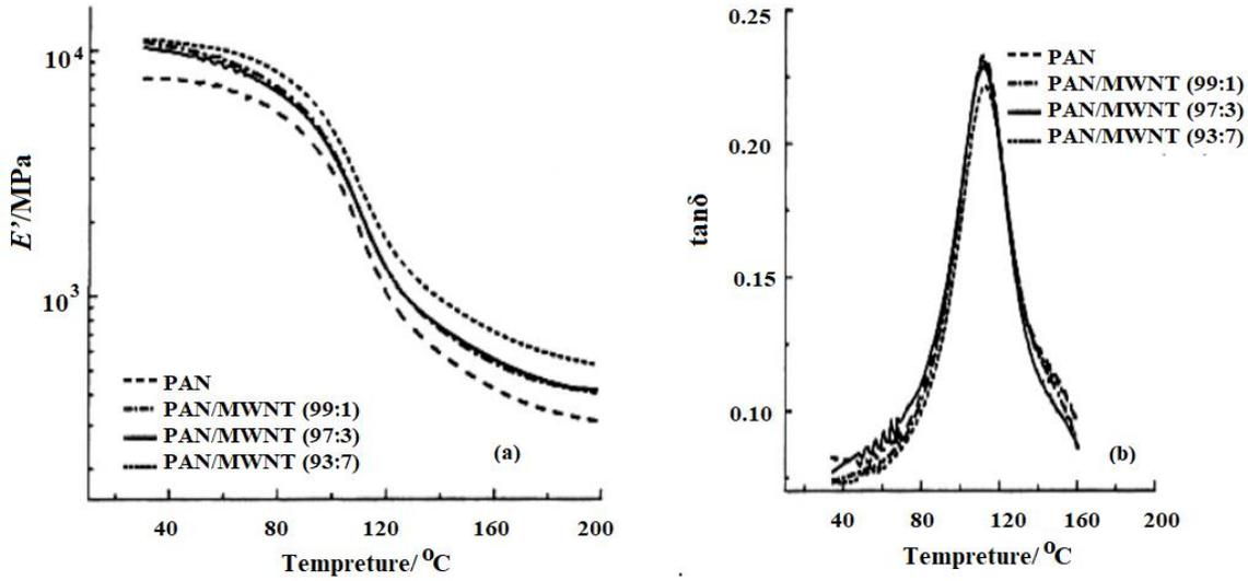
Figure 4. Curves of storage modulus and loss factor versus temperature for PAN / MWNT fibers
