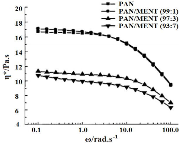
**Figure 1.** Effect of different carbon nanotube content on complex viscosity of PAN/MWNT solution.
