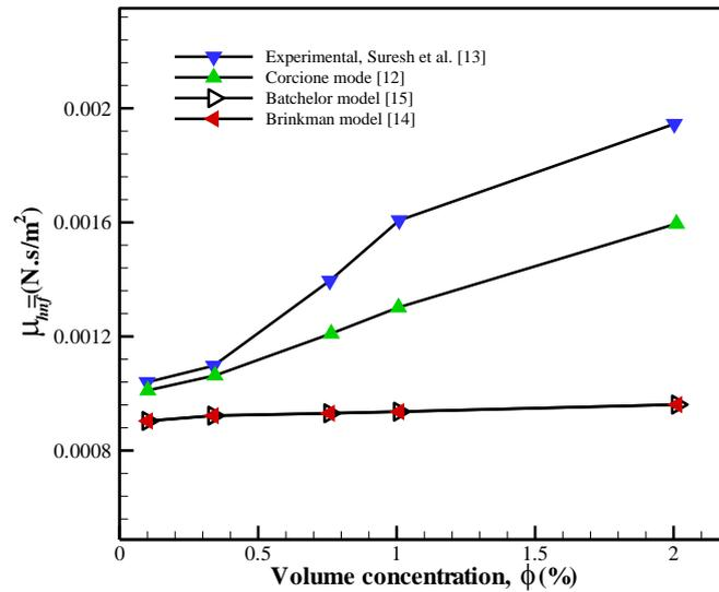
Figure 3: Al2O3-Cu/water hybrid nanofluid Dynamic viscosity.
