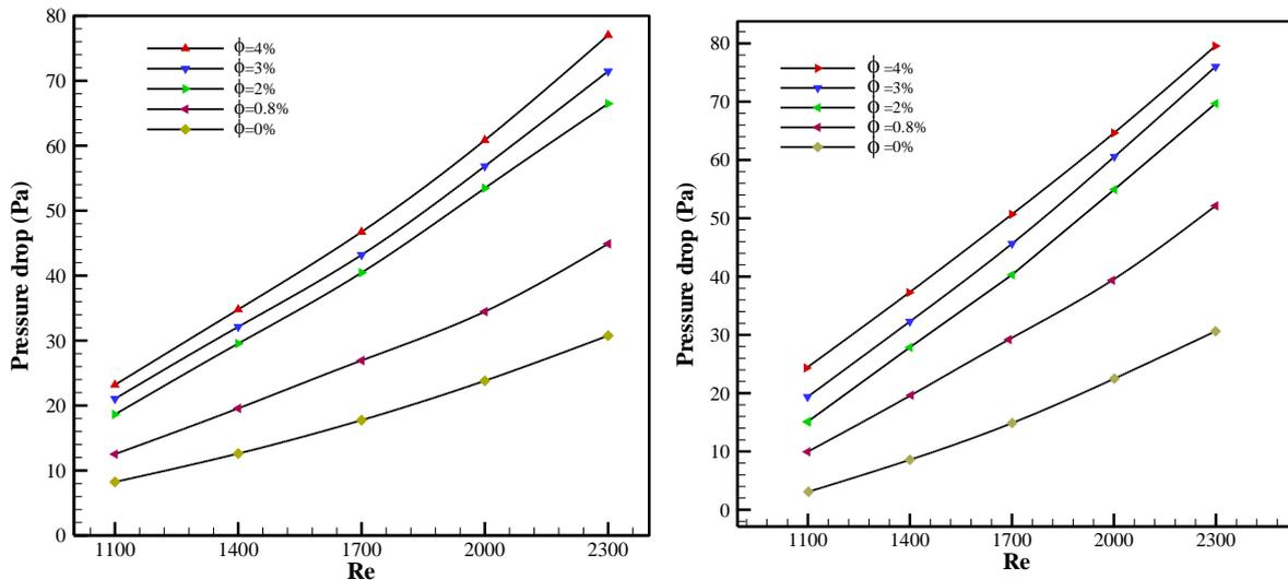
**Figure 10:** Pressure drops Variation vs Reynolds number for diverse volume fractions,  $\phi$  of (a) SiO<sub>2</sub> and (b) MgO/water nanofluid at  $d_p=20\text{nm}$  in the trapezoidal channel.
