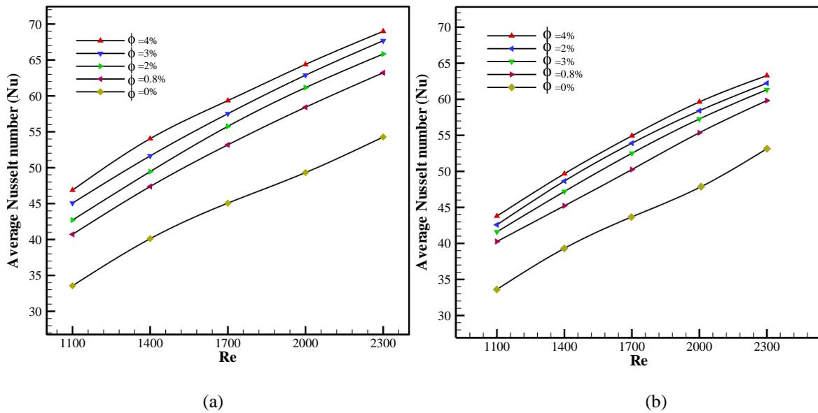
**Figure 9:** Variation of average Nusselt number vs Reynolds number for different volume fractions,  $\phi$  of (a) SiO<sub>2</sub>, and (b) MgO/water nanofluid at  $d_p=20$ nm in the trapezoidal channel.
