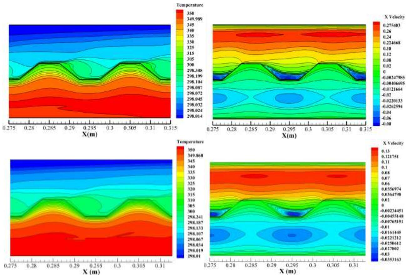
**Figure 6:** streamwise velocity contours and isotherms contours for the trapezoidal-corrugated channel with an amplitude of 4mm and wavelength 20mm at  $Re=1100$ .
