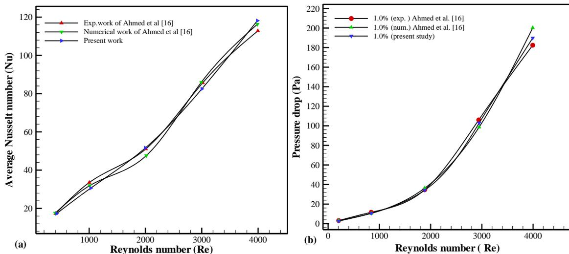
**Figure 5:** Comparison results of turbulent convection in a corrugated channel with Ahmed et al [11]. (a) average Nusselt number versus Reynolds number. (b) pressure drop versus Reynolds number.
