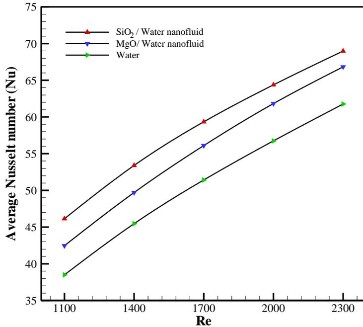
**Figure 7:** Average Nusselt number vs. Reynolds number for different nanoparticles types at  $a=4.0$  mm,  $L_w=20$  mm,  $d_p=20$  nm, and  $\phi=4\%$  in the trapezoidal channel.
