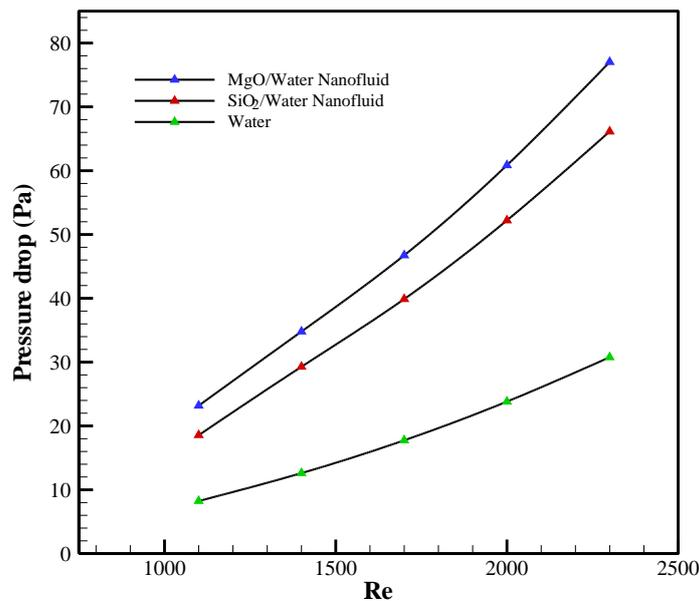
**Figure 8:** Pressure drop vs. Reynolds number for different types of fluids at  $a=4.0$  mm,  $L_w=20$  mm,  $d_p=20$  nm, and  $\phi=4\%$  in the trapezoidal channel.
