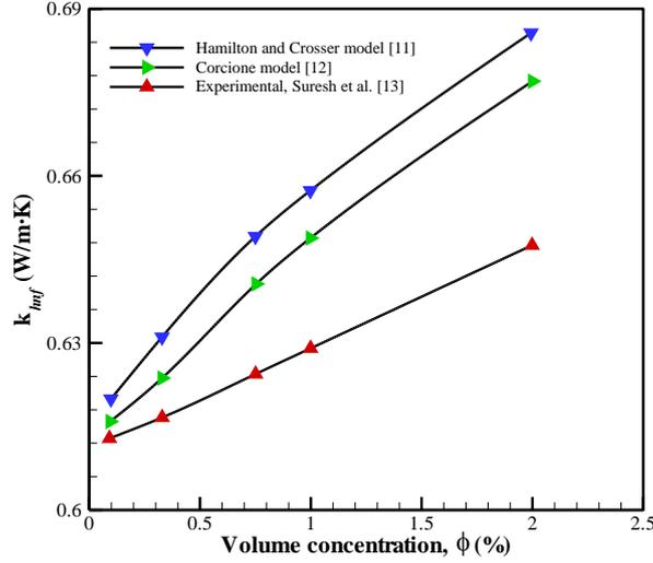
Figure 2: Al<sub>2</sub>O<sub>3</sub>-Cu/water nanofluid Thermal conductivity.
