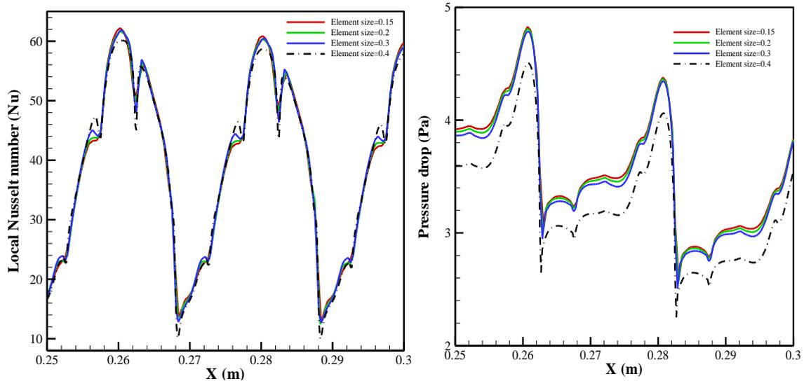
**Figure 4:** (a) local Nusselt number and (b) Pressure drop a long-distance  $X=0.25$  to  $0.3\text{m}$  for water at  $Re = 1200$
