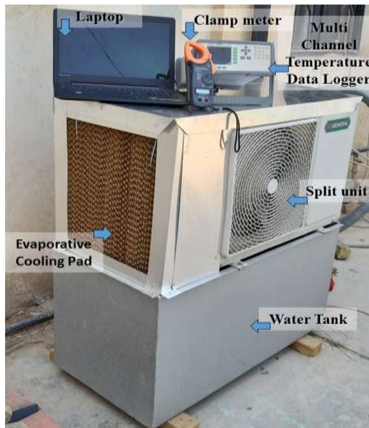
Figure 1: Experimental setup system with measuring device.
