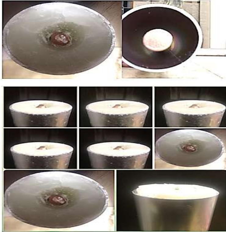
**Figure 4.** Copper rods inside wax-immersed aluminum tubes.
