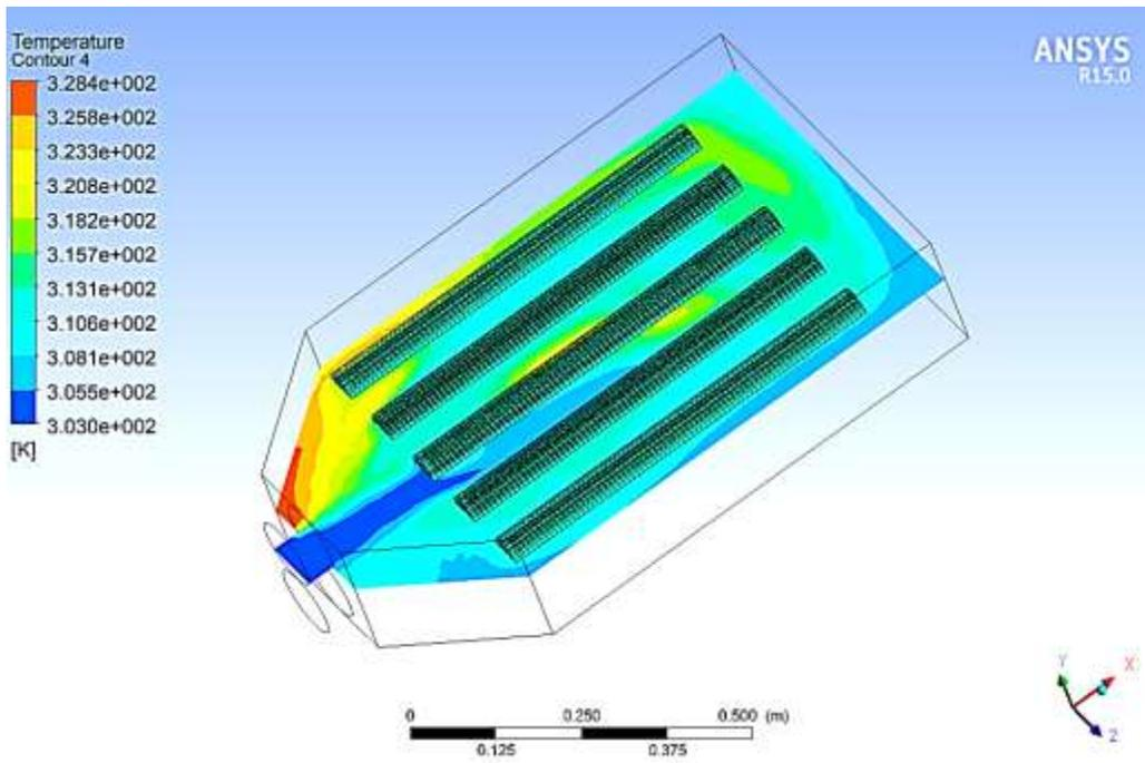
Figure 18. Temperature distribution in the collector.
