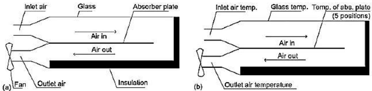
**Figure 7.** (a) Schematic of double pass SAH, (b) Thermocouples locations.
