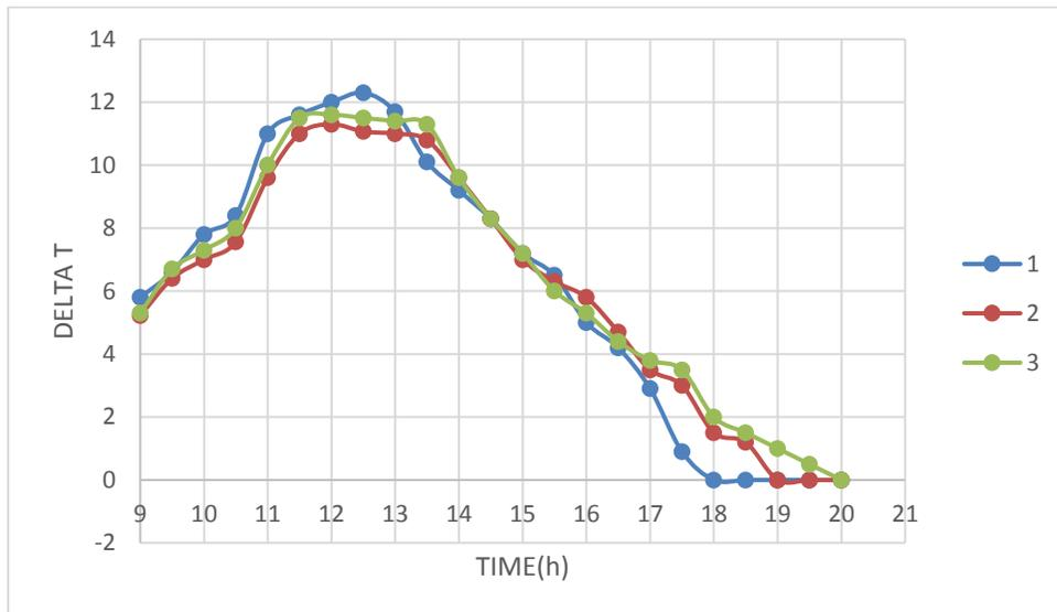
**Figure 14.** Temperature difference (outlet minus inlet) as a function of time for all configurations.
