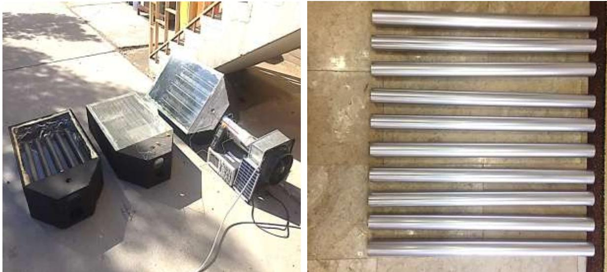
**Figure 1.** Three double pass SAH were fabricated using ten tubes of aluminum.
