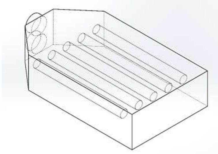
**Figure 8.** Geometry of the solar air heater.
