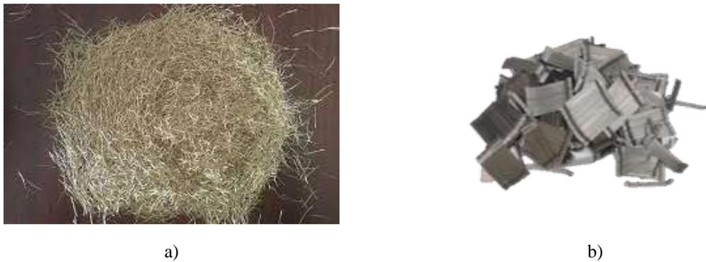
**Figure 1.** Steel fibers used in this study: a) straight type; b) hooked-end type
