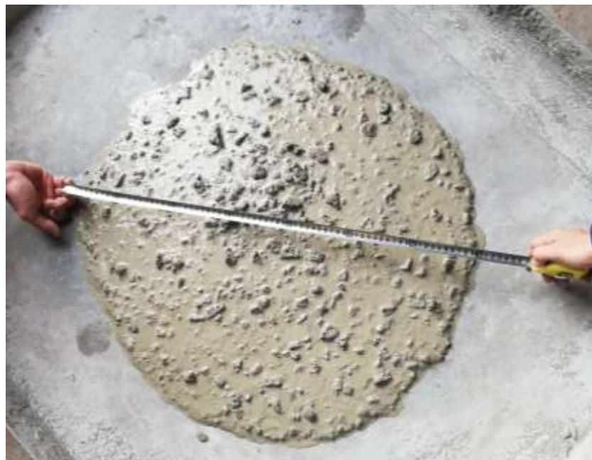
**Figure 2.** Slump-flow test on SFRSCCC mixes with two types of steel fiber at fresh state
