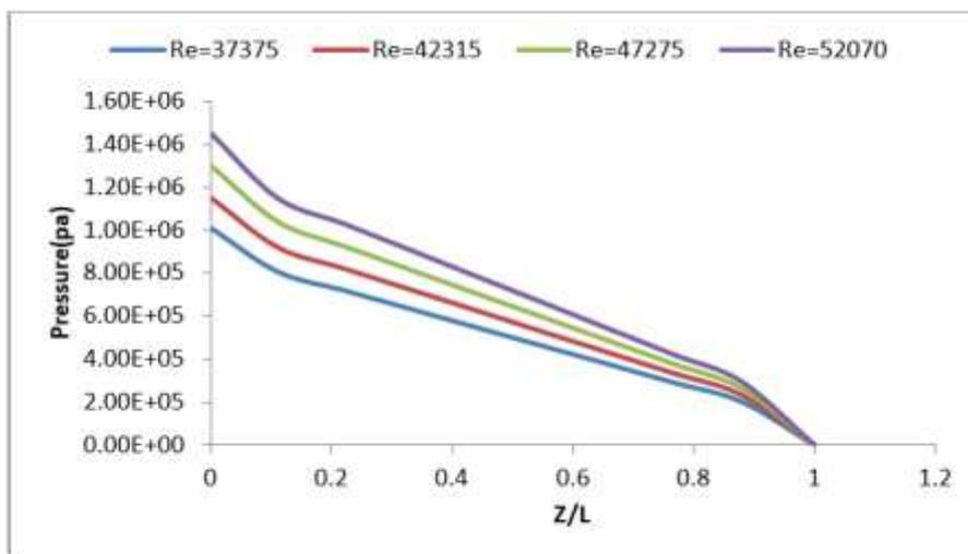
Figure 7. Pressure distribution through porous zone for different Reynolds number
