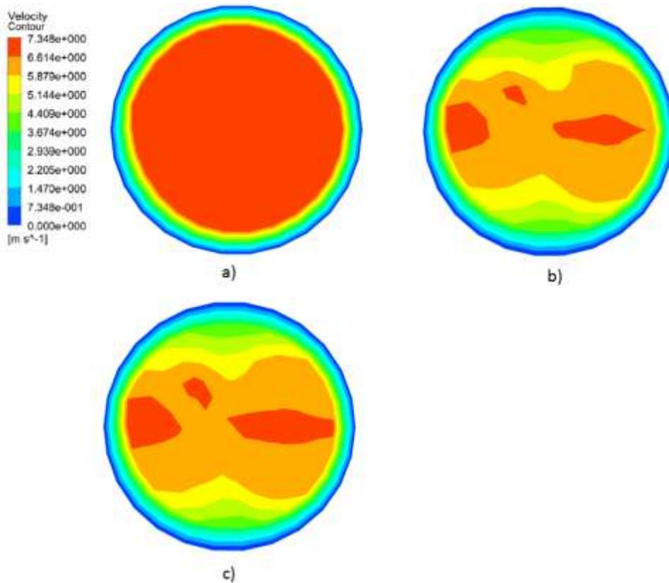
Figure 6. Velocity contour through porous zone at different location (a: inlet, b: mid, c: exit)
