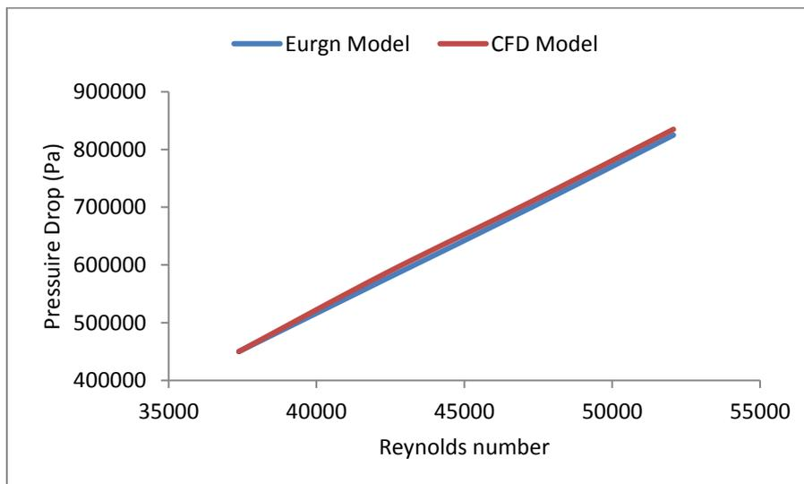
Figure 10. Pressure decreasing through the porous section for different inlet gas velocity
