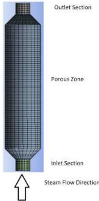
Figure 1. Meshing the test section
