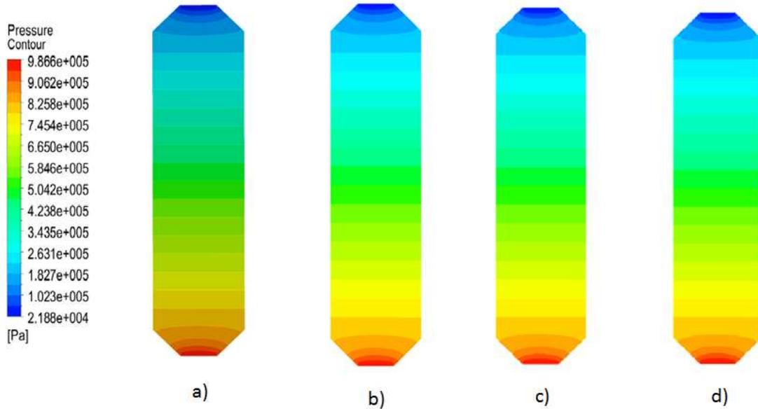
**Figure 2.** Pressure contour through porous zone for different inlet Reynolds number (a: 37375, b: 42315, c: 47275, d: 52070)
