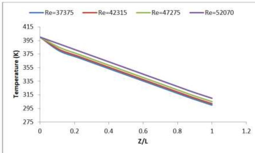
Figure 9. Temperature distribution through porous zone for different Reynolds number
