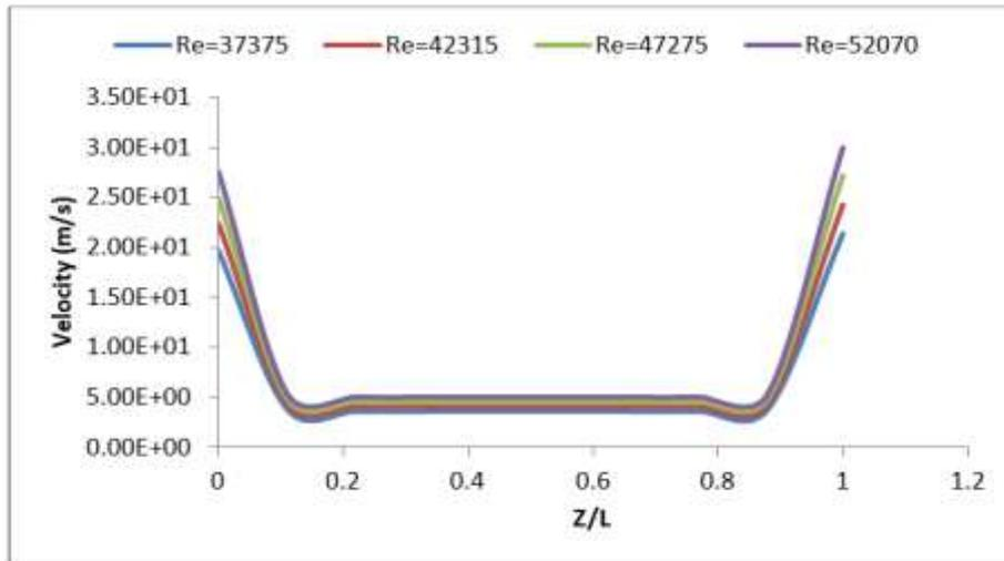
Figure 8. Velocity distribution through porous zone for different Reynolds number
