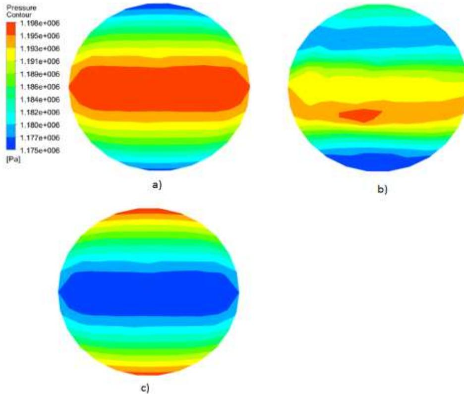
**Figure 5.** Pressure contour through porous zone at different location (a: inlet , b: mid, c: exit, )
