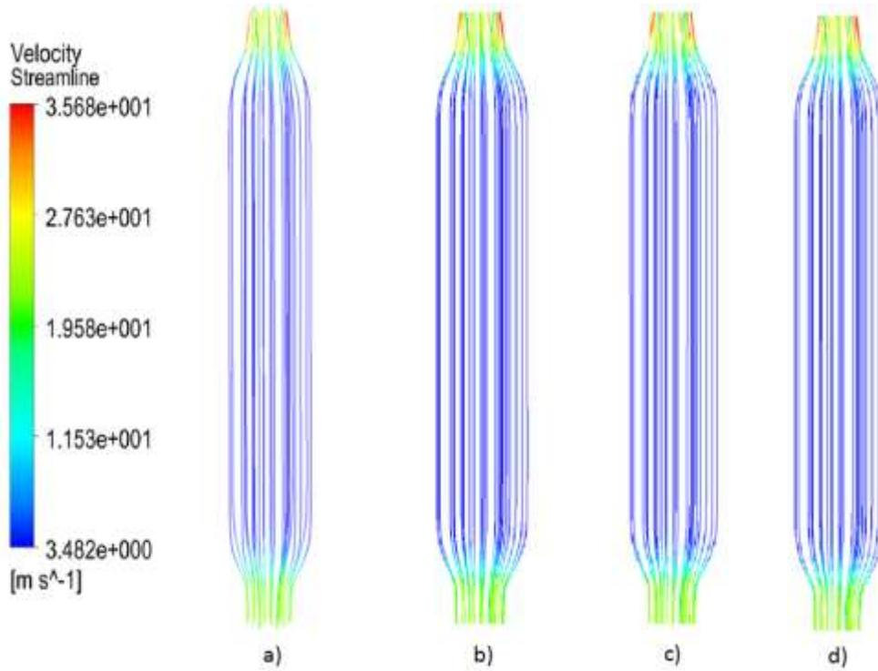
**Figure 4.** Velocity streamline contour through porous zone for different inlet Reynolds number (a: 37375, b: 42315, c: 47275, d: 52070)
