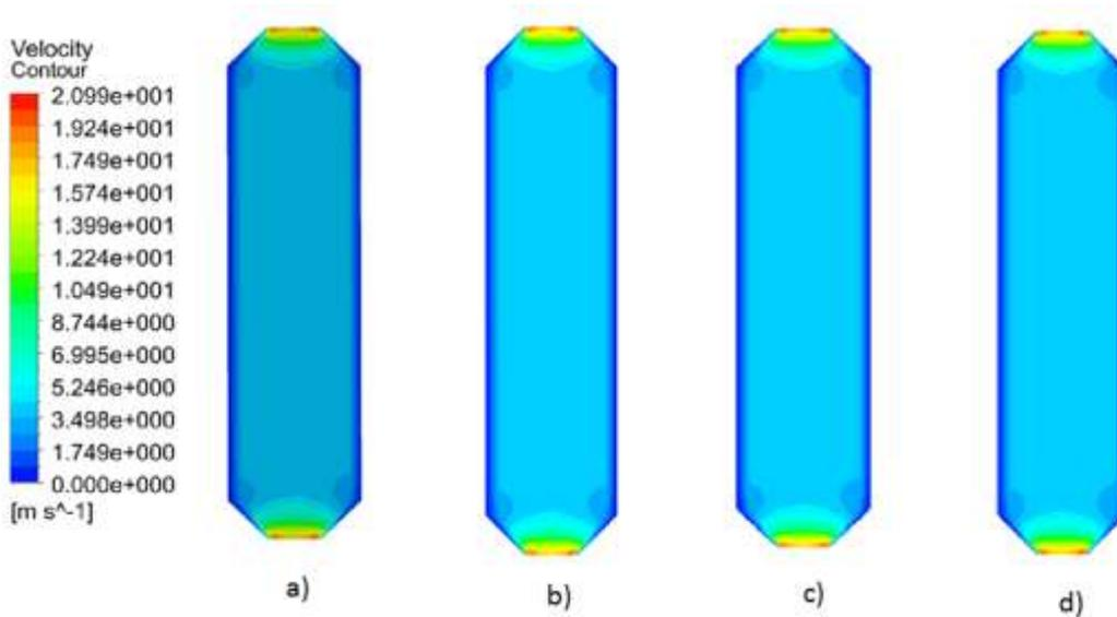
**Figure 3.** Velocity contour through porous zone for different inlet Reynolds number (a: 37375, b: 42315, c: 47275, d: 52070)
