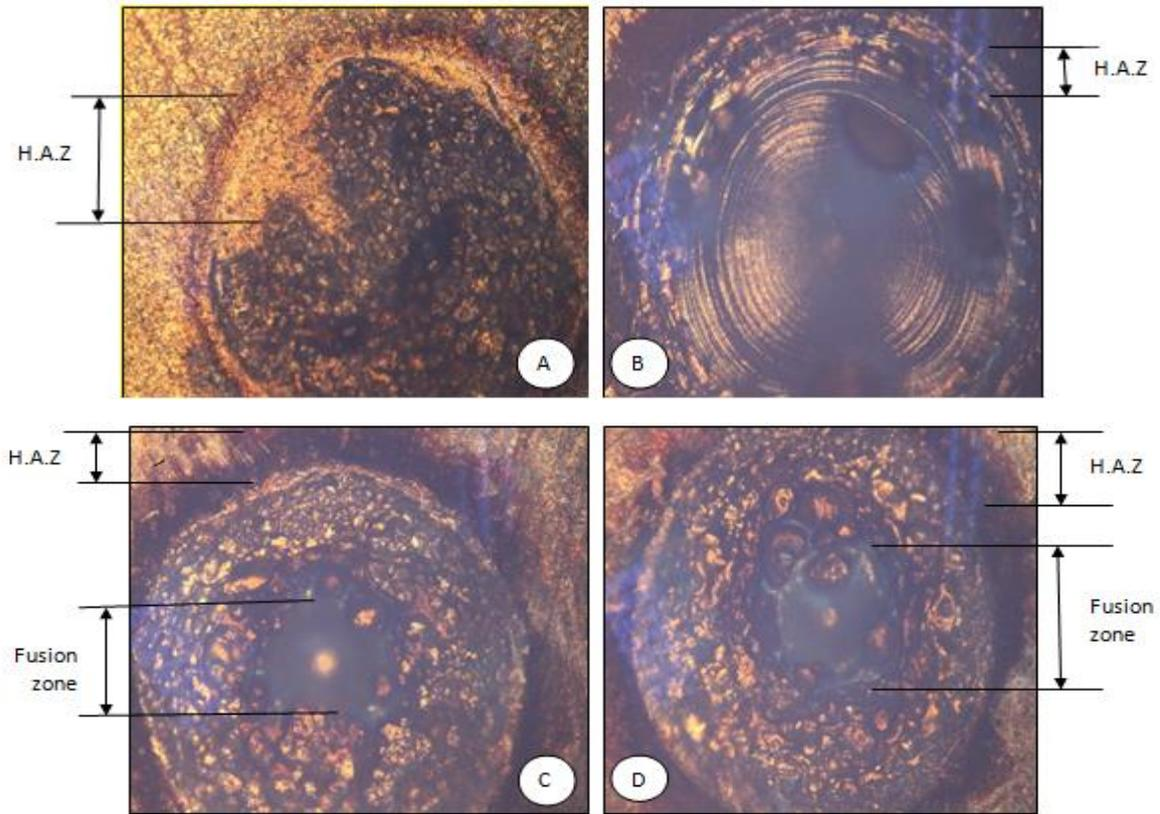
**Figure 5.** shows the molten pool of carbonitriding steel after laser melting with different energies and pulse duration (A: 0.89J with 1ms), (B: 2J with 2.33ms), (C: 4Jwith 4.47 ms),(D:9J with 9.87ms).
