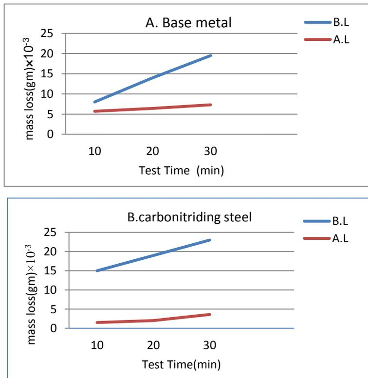
**Figure 6.** shows the relationship between the mass loss and the period time.A: base metal and B: carbonitriding g steel, B.L (befor laser), A.L (after laser).
