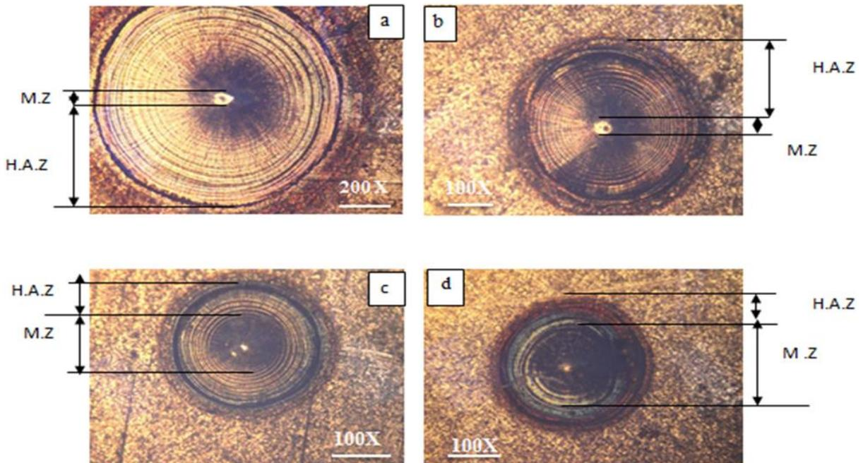
**Figure 4.** shows the molten pool of base metal after laser melting with different energies and pulse duration (A: 0.89J with 1ms), (B: 2J with 2.33ms), (C: 4Jwith 4.47 ms),(D:9J with 9.87ms).
