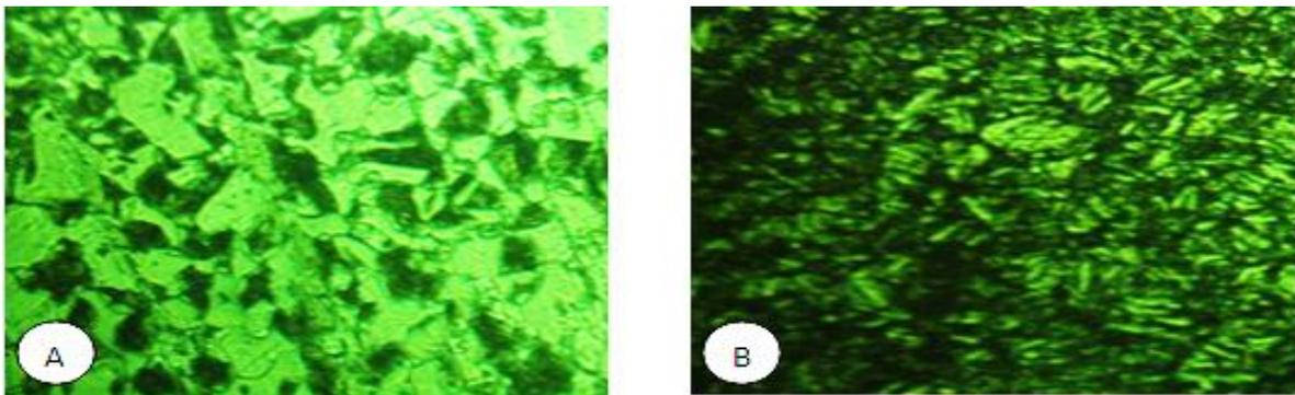
**Figure 2.** Micro structure of samples, A: base metal and B: after carbonitriding at 40X.
