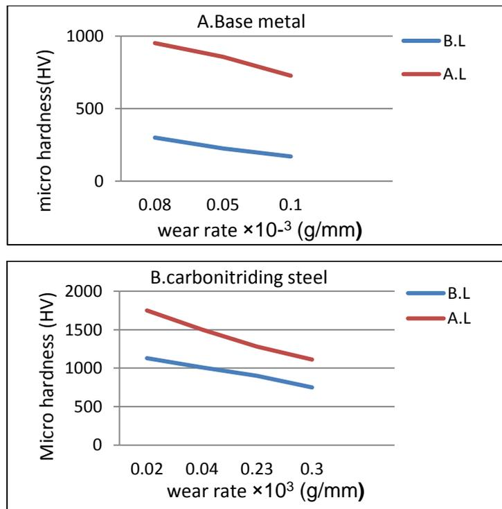
**Figure 8.** shows the relationship between the wear rate and micro hardness. A: base metal and B: carbonitriding steel, B.L (befor laser), A.L (after laser).
