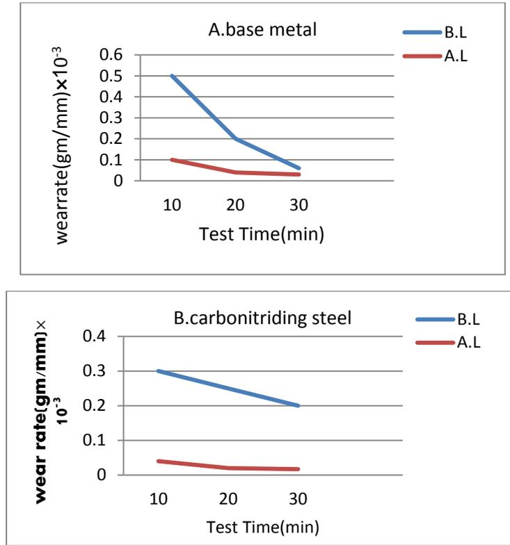
**Figure 7.** shows the relationship between the wear rate and the period time. A: base metal and B: carbonitriding steel, B.L (befor laser), A.L (after laser).
