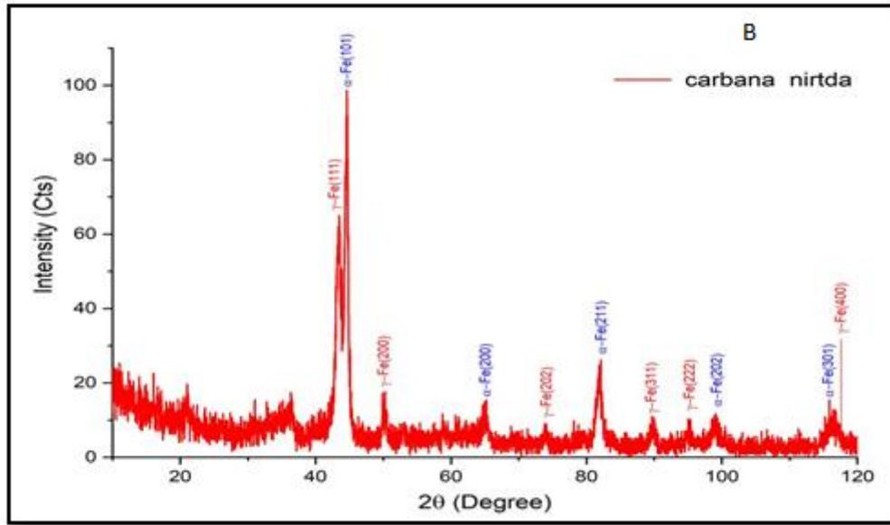
**Figure 3.** X-Ray diffraction of specimens, A; base metal and B; after carbonitriding
