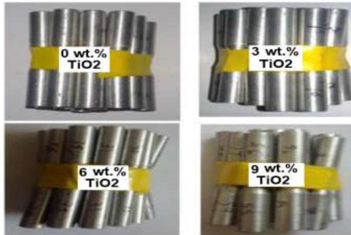
**Figure 2.** Nanocomposite specimens after production for TiO<sub>2</sub>
