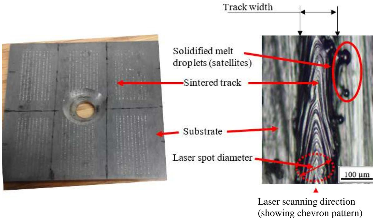
**Figure 2.** Top view of the substrate and the single tracks.
