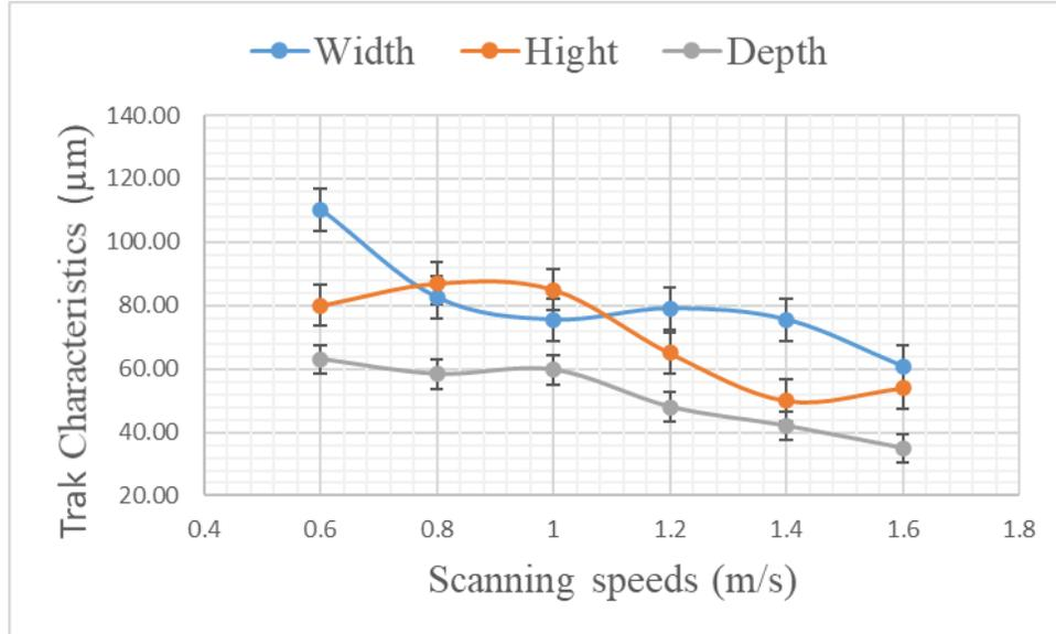
**Figure 3.** Tracks characteristics at 150 W as a function of scanning speeds
