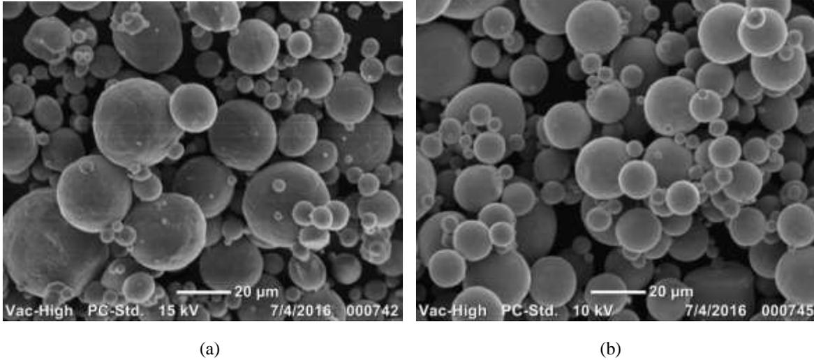
**Figure 1.** SEM image of the supplied powders (A) CpTi (B) Mo
