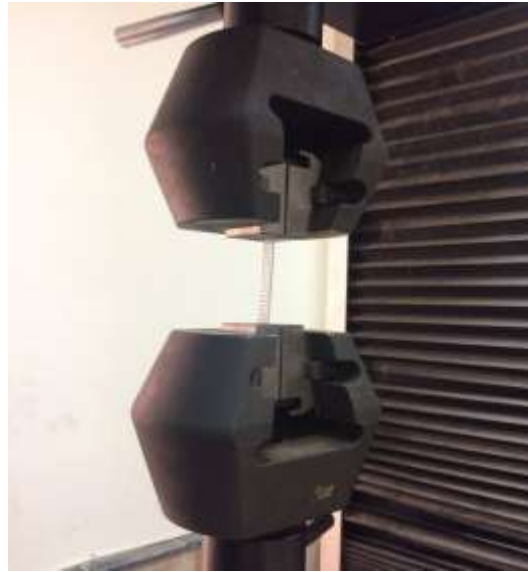
Figure 2. Tensile specimen fixed on universal testing machine.
