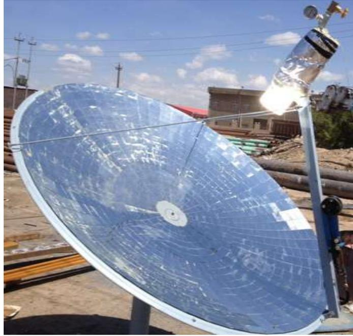
**Figure 3.** Experimental setup of PDC for 2<sup>nd</sup> model.
