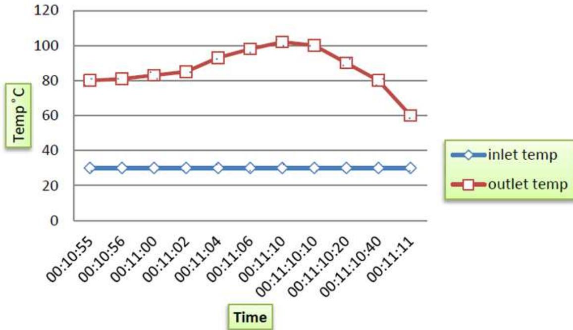
Figure 4. Temperature variation for nickel sheet metal reflector with radiator heat exchanger receiver tank for April.
