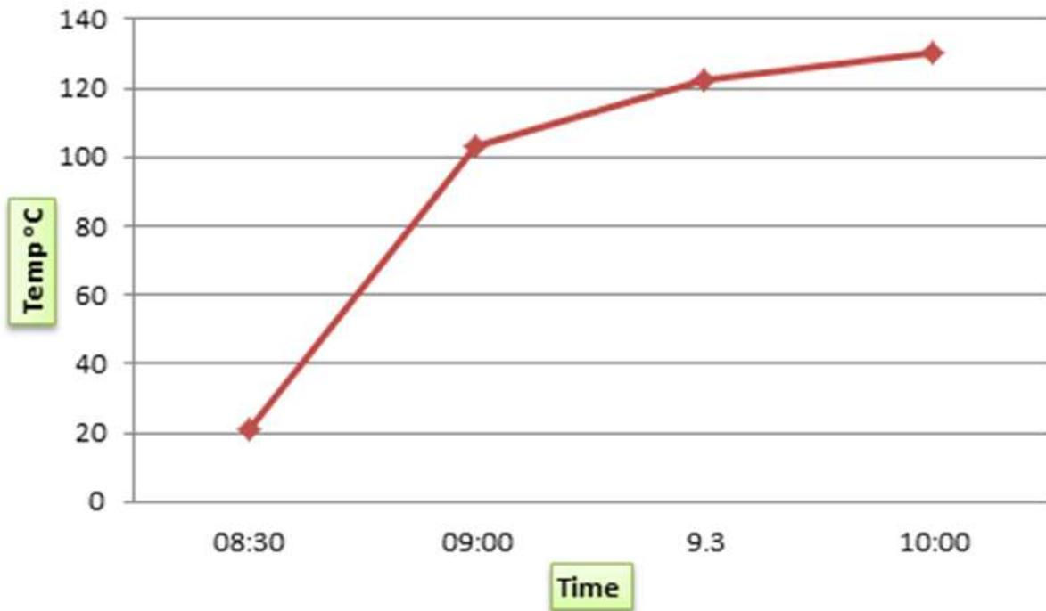
Figure 7. Outlet temperature variation for mirror reflector with cylindrical vessel receiver tank for April.
