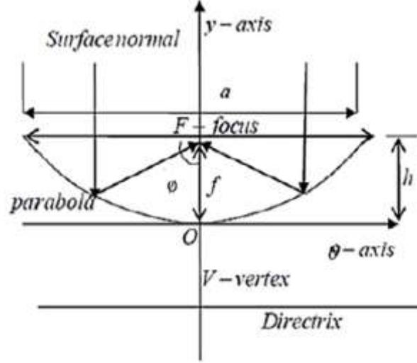
**Figure 1.** Dimensions and geometry of the solar collector parabolic dish.
