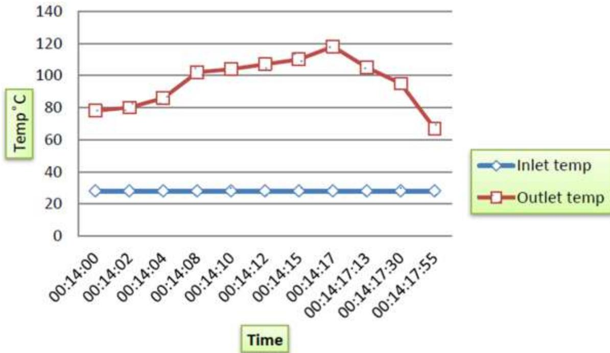
Figure 5. Temperature variation for nickel sheet metal reflector with radiator heat exchanger receiver tank for April.
