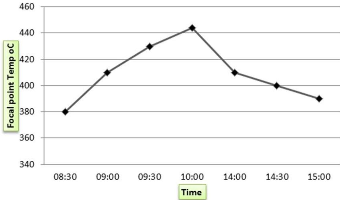
Figure 10. Focal point temperature for mirror reflector with cylindrical vessel receiver tank for April.
