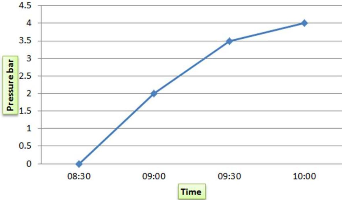
Figure 9. Pressure variation for mirror reflector with cylindrical vessel receiver tank for April.
