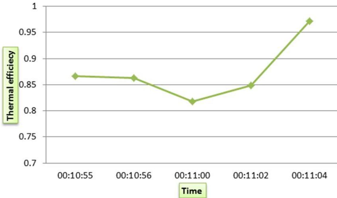
Figure 6. Thermal efficiency with time for nickel sheet metal reflector with radiator heat exchanger receiver tank for April.
