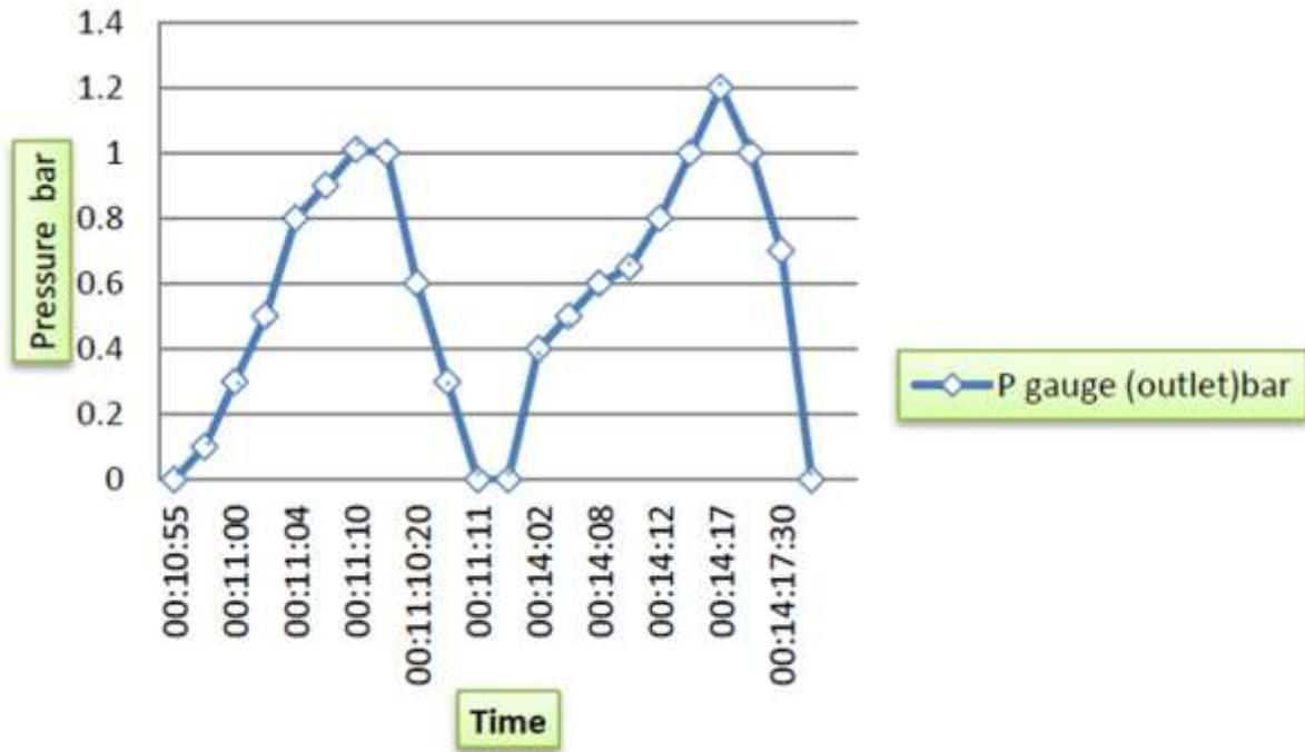
Figure 5. Pressure variation for nickel sheet metal reflector with radiator heat exchanger receiver tank for April.
