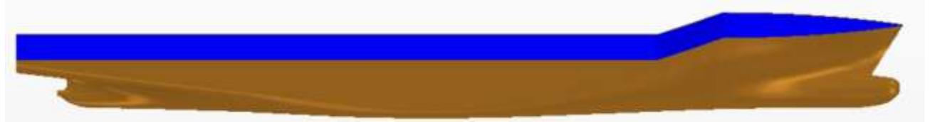
**Figure 1.** Geometry of KCS containership [23]
